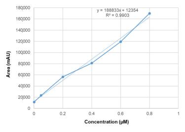
**Figure 1.** Analytical curve of the HPLC-TBARS-EVSC assay in the range of 0.001 to 0.8  $\mu$ M, with line equation y = 188,833x + 12,354.
