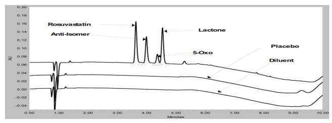
Fig. 2. Overlaid chromatograms of placebo, diluent and standard (for identification)
