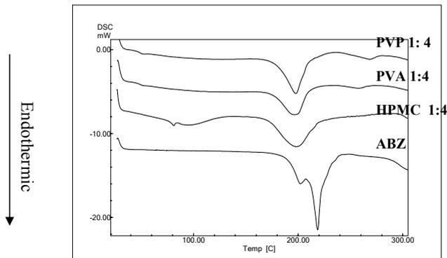
**Fig. 4.** DSC curves of ABZ alone and its physical mixtures with HPMC, PVA, and PVP in 1:4 ratios
