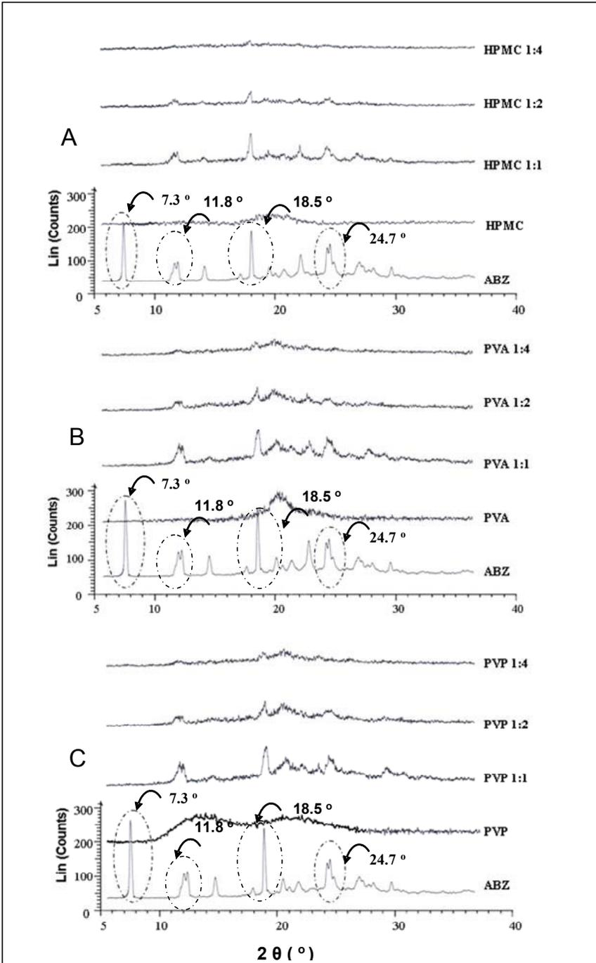
**Fig. 5.** Powder X-ray diffraction patterns of albendazole as well as HPMC microparticles (A), PVA microparticles (B), and PVP microparticles (C)
