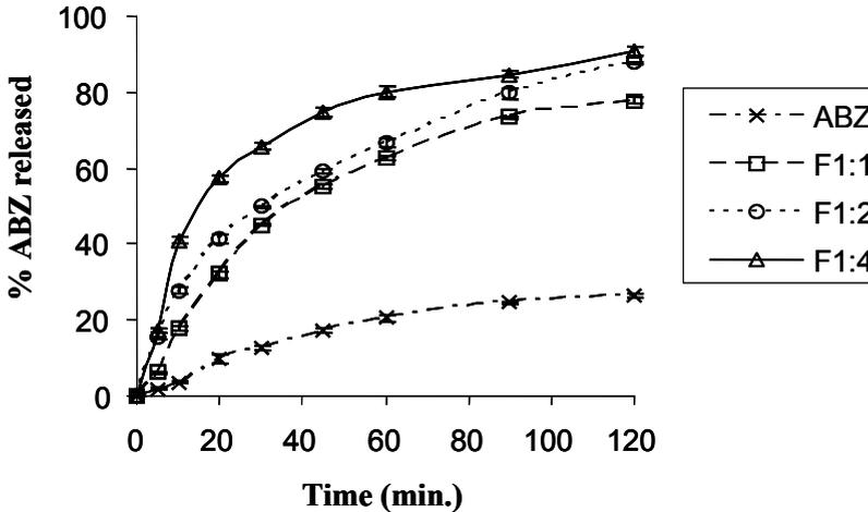
**Fig. 7.** Dissolution profiles of ABZ–PVA microparticles in pH 1.2 at  $37 \pm 0.5 \text{ }^\circ\text{C}$  prepared by spray drying technique. Each point represents the mean  $\pm$  standard deviation of three experiments ( $P < 0.05$ ).
