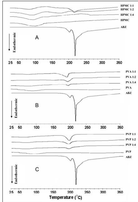
**Fig. 3.** DSC thermograms of albenzazole as well as HPMC microparticles(A), PVA microparticles (B), and PVP microparticles (C)
