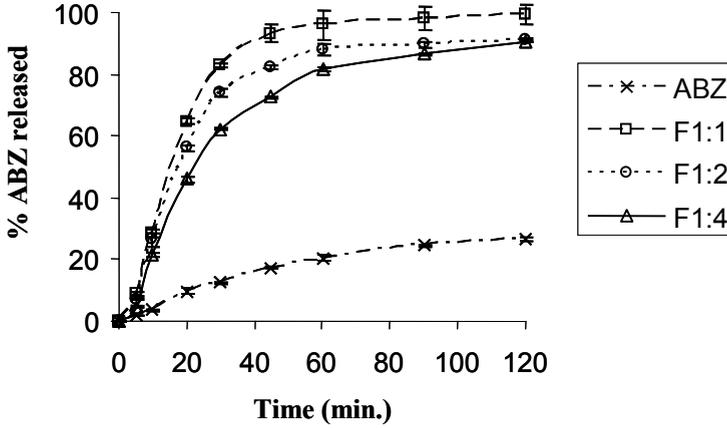
**Fig. 6.** Dissolution profiles of ABZ–HMPC microparticles in pH 1.2 at  $37 \pm 0.5 \text{ }^\circ\text{C}$  prepared by spray drying. Each point represents the mean  $\pm$  standard deviation of three experiments ( $P < 0.05$ ).
