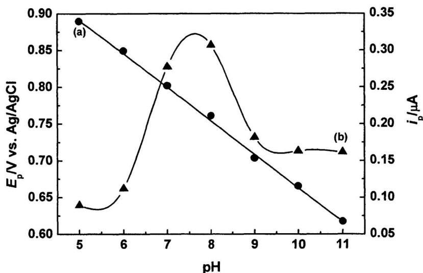
**Fig. 2.** Effect of pH on (a) peak potential and (b) peak current in Britton–Robinson buffer using differential pulse voltammetry at glassy carbon electrode. Loperamide hydrochloride concentration,  $1.0 \times 10^{-5}$  M; scan rate, 10 mVs $^{-1}$ ; pulse amplitude, 50 mV; pulse width, 30 s
