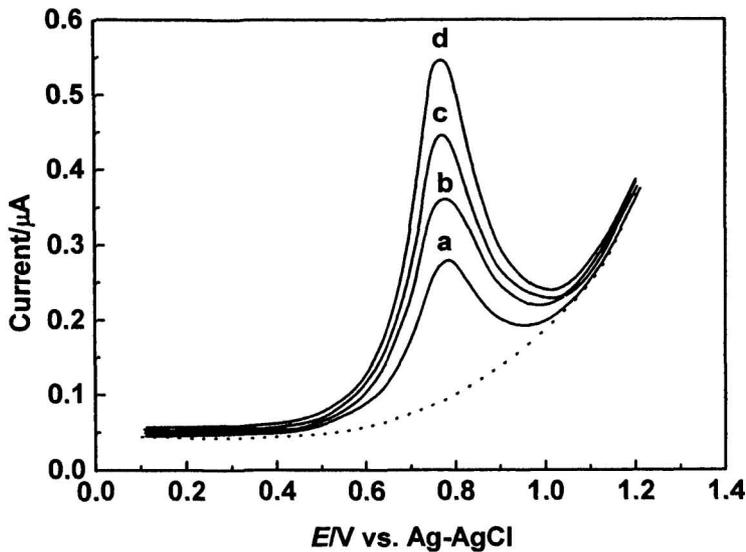
**Fig. 4.** Differential pulse voltammograms for increasing concentrations of loperamide hydrochloride in Britton–Robinson buffer at pH 8.0 on glassy carbon electrode. Scan rate, 10 mVs.1; pulse amplitude, 50 mV; pulse width, 30 ms. Loperamide hydrochloride concentration: (1)  $7.5 \times 10^{-6}$  M, (2)  $1.5 \times 10^{-5}$  M, (3)  $2.25 \times 10^{-5}$  M and (4)  $3.0 \times 10^{-5}$  M; the dotted lines represent blank solution.
