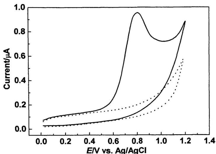
**Fig. 3.** Cyclic voltammograms of  $5.0 \times 10^{-4}$  M loperamide hydrochloride solution on glassy carbon electrode in Britton–Robinson buffer at pH 8.0. Scan rate,  $100 \text{ mVs}^{-1}$ . The dotted lines represent blank solution
