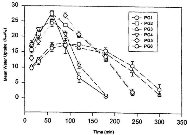
Fig. 1b. Water uptake of CMC based patches with Propylene glycol as plasticizer
