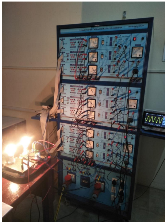
Figure 52. Hardware setup for seven-level cascade inverter at Shanmugha Arts, Science, Technology & Research Academy (SASTRA).
