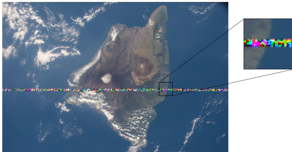
Figure 2. Detailed view of a corrupted demosaicked image when the stored Bayer image is affected by a band SEFI.
