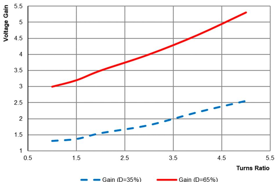
**Figure 20.** Voltage gain dependency on duty cycle and turns ratio between L<sub>1</sub>, L<sub>2</sub>, and L<sub>3</sub>, while L<sub>1</sub> = L<sub>2</sub>.
