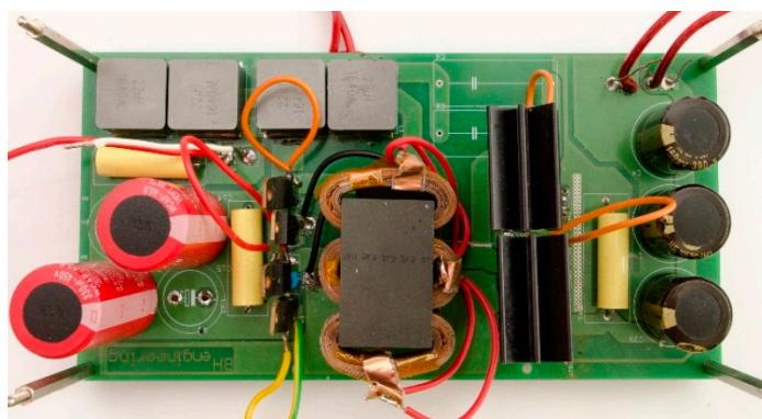
**Figure 12.** Proposed converter prototype.
