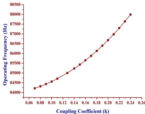
Figure 13. Operating frequency corresponding to coupling coefficient.
