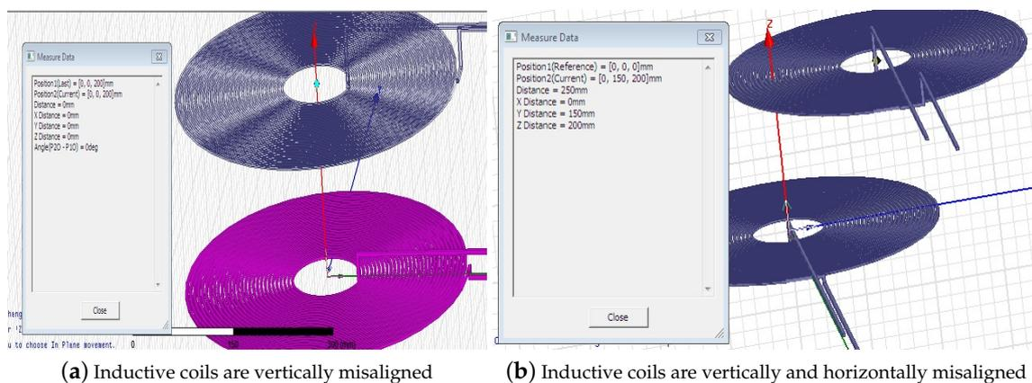
(a) Inductive coils are vertically misaligned
