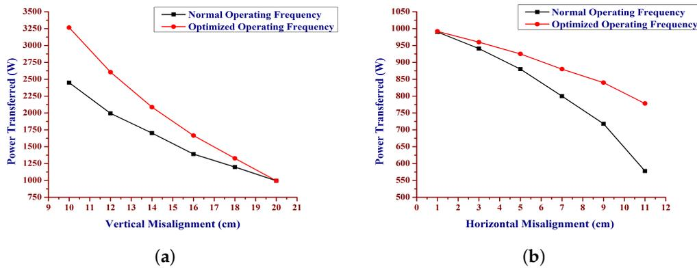
**Figure 15.** Power transfer level corresponding to the misalignment. (a) Power transferred corresponding to the vertical misalignment. (b) Power transferred corresponding to the horizontal misalignment.
