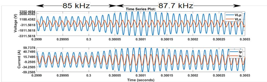
Figure 12. Voltage and current waveform of inductive track at  $M = 25 \mu\text{H}$  while tuning.
