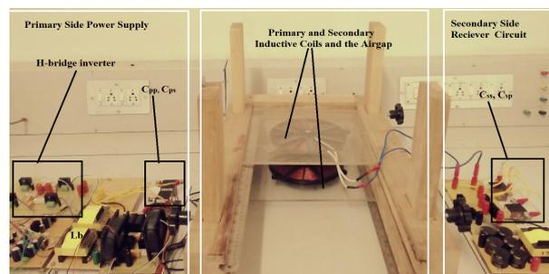
**Figure 17.** Experimental prototype of LCL architecture.
