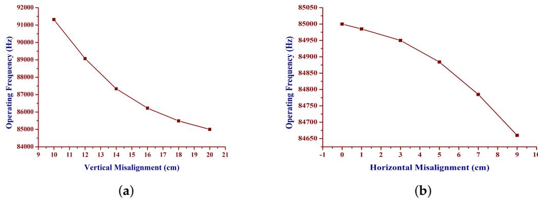
**Figure 14.** Operating frequency corresponding to misalignment. (a) Operating frequency corresponding to the vertical misalignment. (b) Operating frequency corresponding to the horizontal misalignment.
