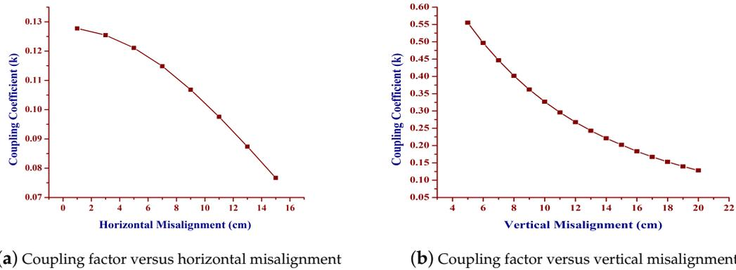
Figure 7. Coupling factors for various misalignments.
