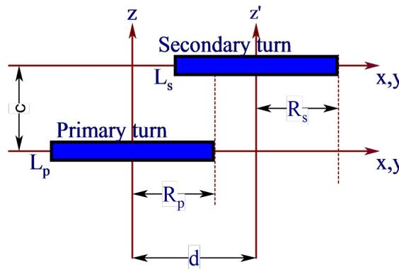
Figure 4. Circular coils with vertical and horizontal misalignment.
