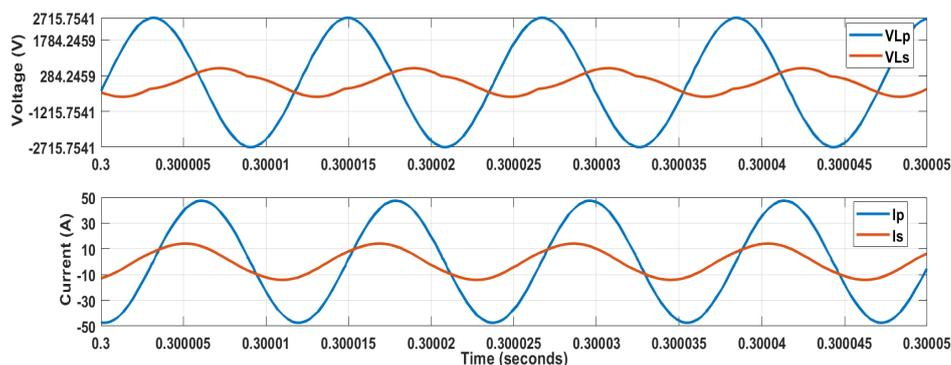
Figure 10. Voltage and current waveform of the inductive track at  $M = 14 \mu\text{H}$  and  $f = 85 \text{ kHz}$ .
