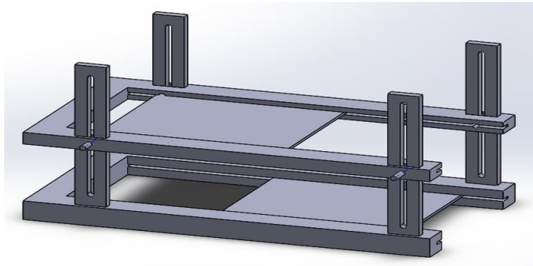
Figure 8. Dynamic structure of the IPT coil plates.
