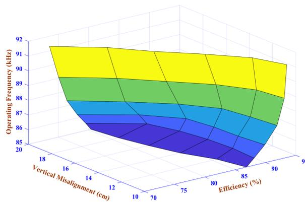
Figure 18. Power transfer efficiency against to the vertical misalignment and operating frequency.
