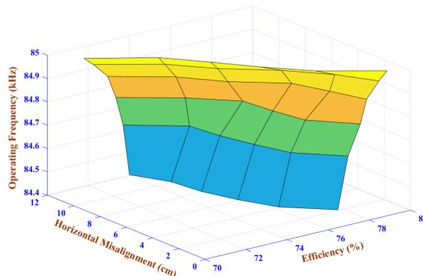
Figure 19. Power transfer efficiency against to the horizontal misalignment and operating frequency.
