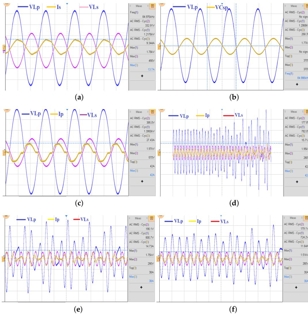
**Figure 16.** Experimental waveforms. (a) Voltage  $V_{Lp}$ , current  $I_s$ , and voltage  $V_{Ls}$ . (b) Voltage  $V_{Lp}$  and  $V_{Csp}$ . (c) Steady state voltage and current waveform. (d) AC transients, due to horizontal misalignment. (e) AC transients, due to horizontal and vertical misalignment. (f) AC transients, due to minor perturbations of the coil.
