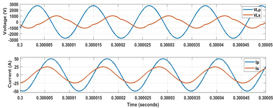
Figure 11. Voltage and current waveform of the inductive track at  $M = 25 \mu\text{H}$  and  $f = 87.7 \text{ kHz}$ .
