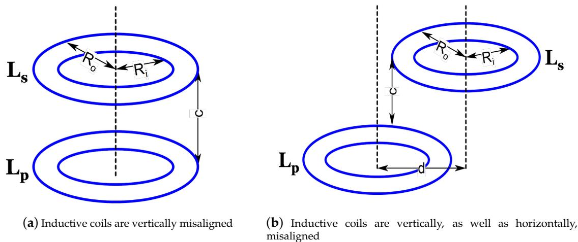
Figure 3. Misalignment of inductive coil.
