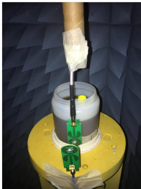
**Figure 4.** Position of the bone marrow lesion phantom inside the anechoic chamber. The phantom was placed in the centre of a rotatable table. The external PulsON P200 antenna is the transmitter, and the internal PulsON P200 antenna is the receiver.
