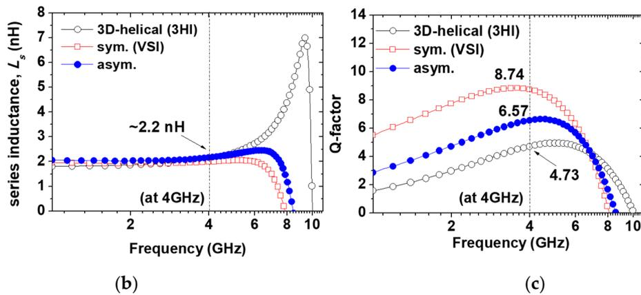
Figure 1. (a) Representation of three different types (conventional, VSI, and 3HI) of inductors with same inductance of 2.2 nH. (b) Measured series inductance ( $L_s$ ) and (c) their Q-factors at 4 GHz.
