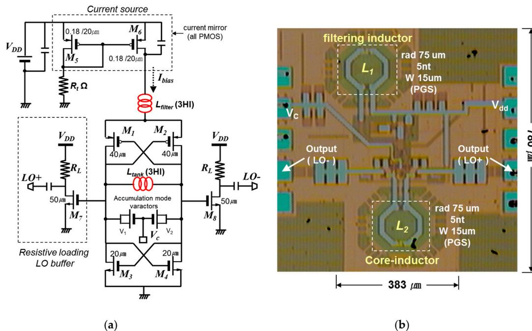
Figure 3. (a) Designed LC-VCO schematic diagram. (b) Chip microphotograph ( $0.283 \times 0.623 \text{ mm}$ ).
