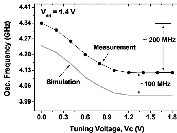
Figure 5. Comparisons between measured and simulated results.
