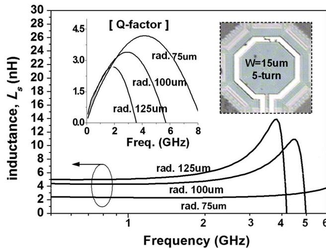
Figure 2. Measured inductance ( $L_s$ ) and Q-factors of fabricated symmetric helical inductors.
