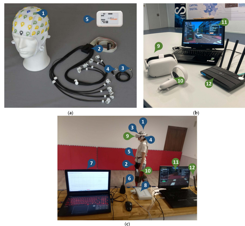
Figure 2. The EEG and VR equipment: (a) Main components of the EEG recorder kit; (b) Main components of the VR equipment; (c) The final setup worn by participants during the experiments. Readers may refer to Table 1 for the description and numbering of components.
