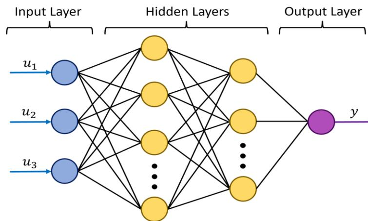
**Figure 7.** Structure of an ANN with the input, hidden, and output layers.
