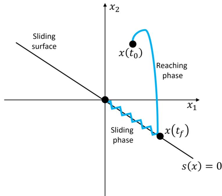
**Figure 4.** Schematic of the sliding surface of an SMC strategy.
