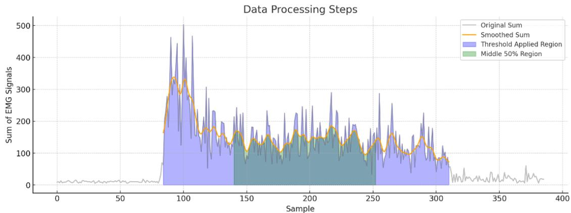
Figure 7. Data extraction illustration for a stable force curve.
