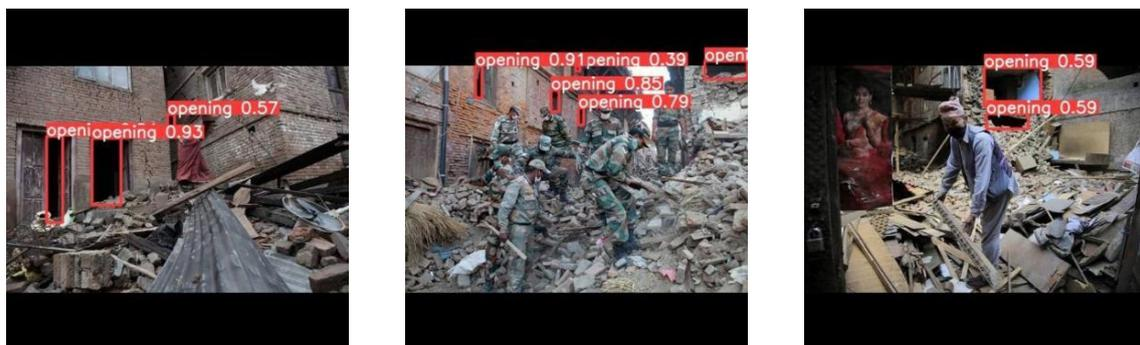
**Figure 4.** YOLOv5s detection output on the test dataset. Openings such as open doors, windows, and collapsed walls were successfully detected.
