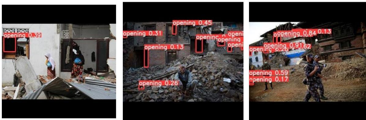
**Figure 5.** YOLOv5s detection output on the test dataset. False negatives and false positives were detected.
