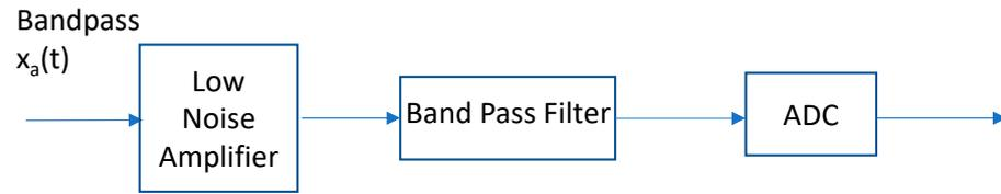
Figure 4. Direct bandpass sampling without mixers.
