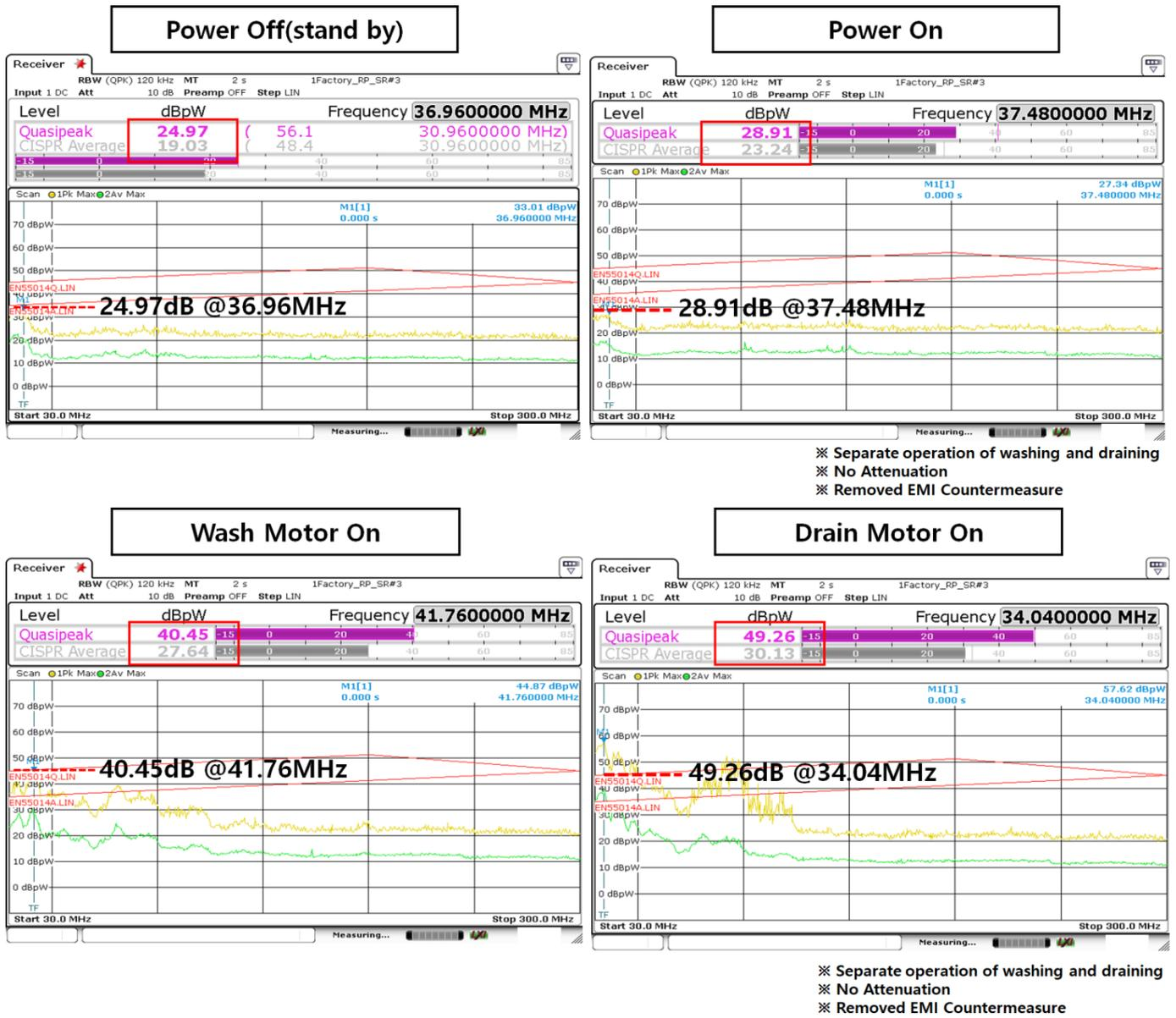
Figure 17. EMI (RP) results based on each load operation status.
