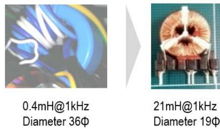
Figure 23. Harness core changed to PCB mounting type.
