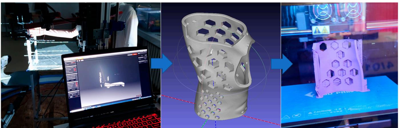
**Figure 6.** Customized therapeutic orthosis design and production for the purpose of VR system prototyping.
