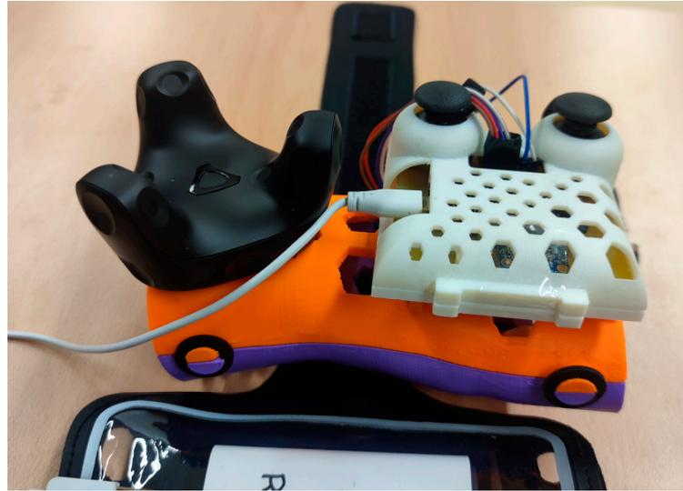
**Figure 11.** Assembled orthosis with controller, motion tracker, straps, and powerbank.
