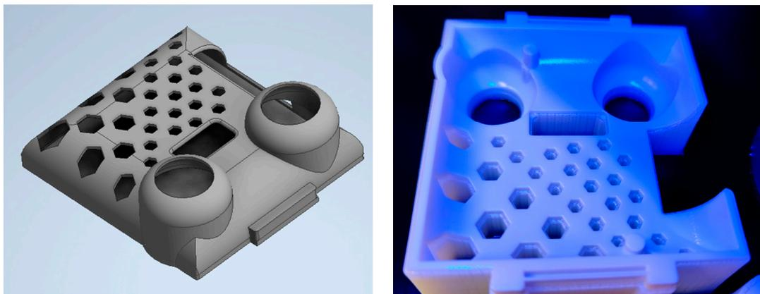
**Figure 8.** Housing of the controller—design and production.
