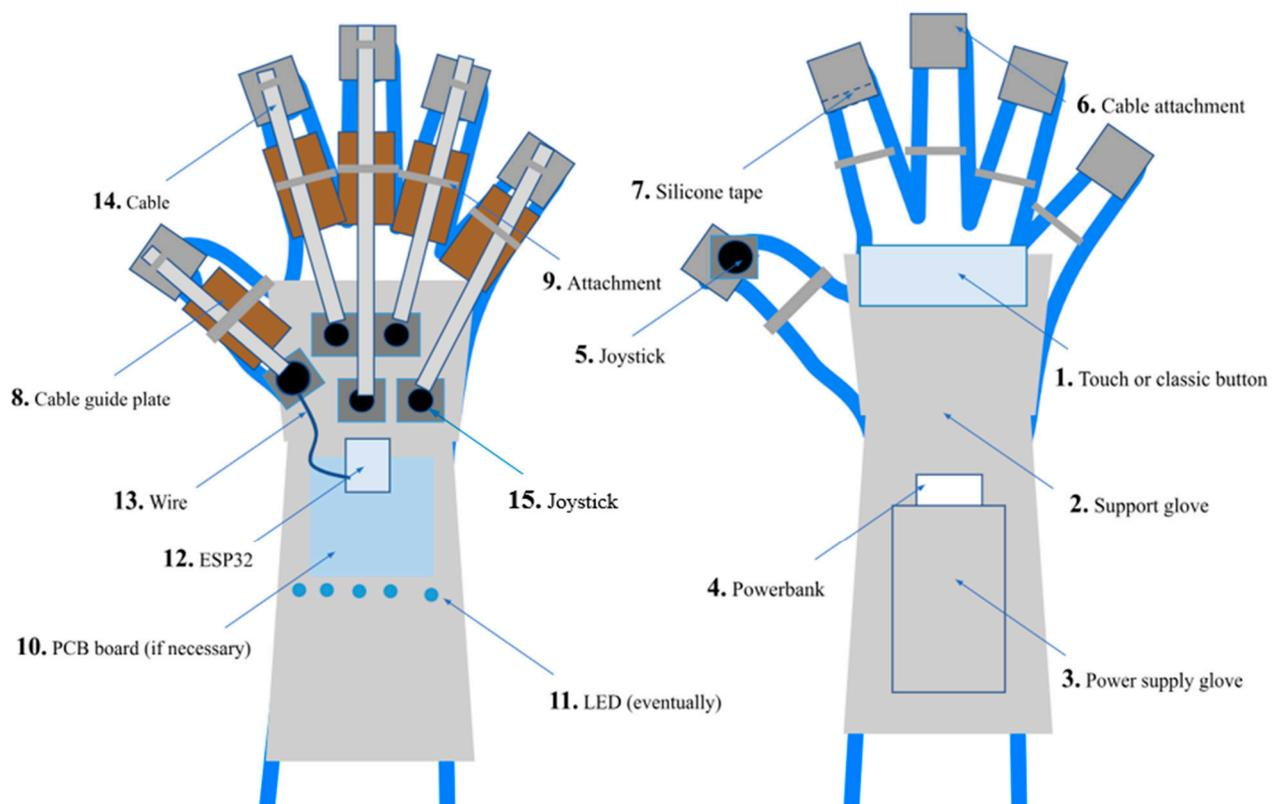
**Figure 7.** Controller schematic, indicating the most important components.
