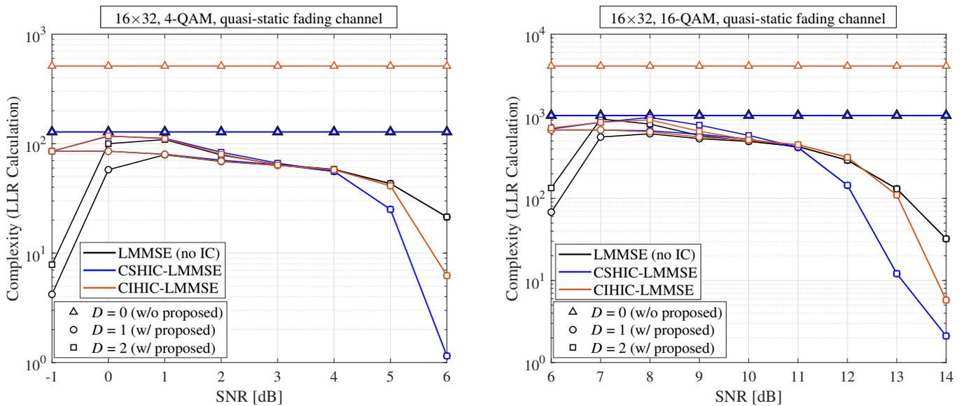
**Figure 18.** The complexity of LLR calculation per receive signal vector for  $16 \times 32$  MMARQ systems with LMMSE under the quasi-static fading channel.
