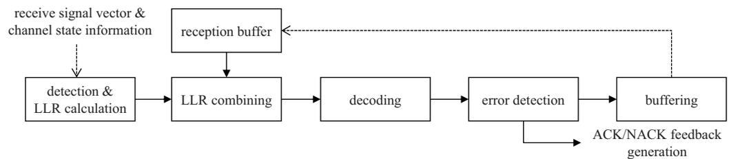
Figure 2. The reception procedure of the linear detection-based receiver.
