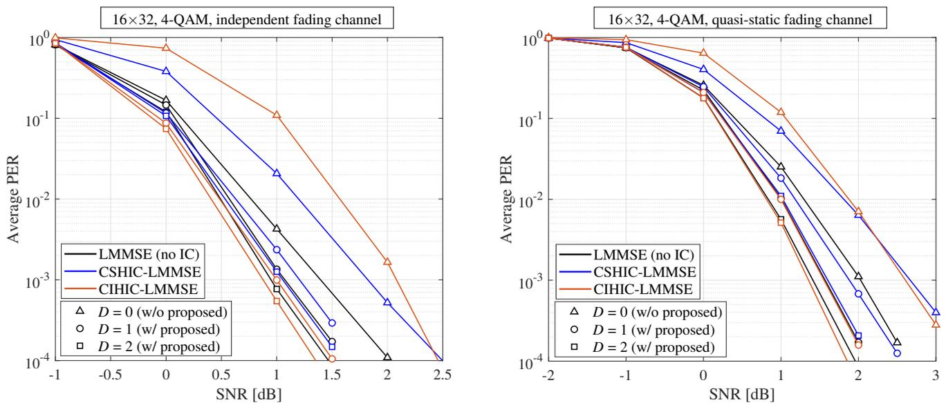
Figure 6. The average PERs for  $16 \times 32$  MMARQ systems with LMMSE and 4-QAM.
