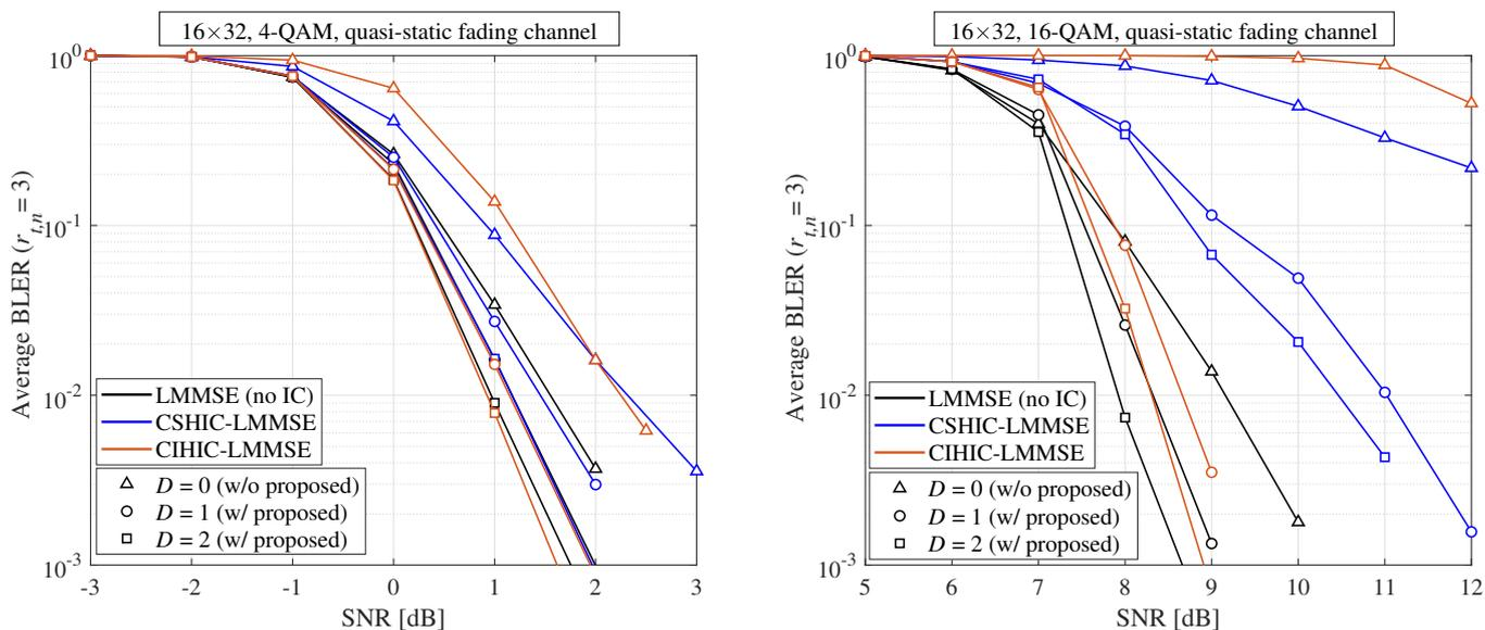
**Figure 12.** The average BLERs of 3rd HARQ round for  $16 \times 32$  MMARQ systems with LMMSE under the quasi-static fading channel.
