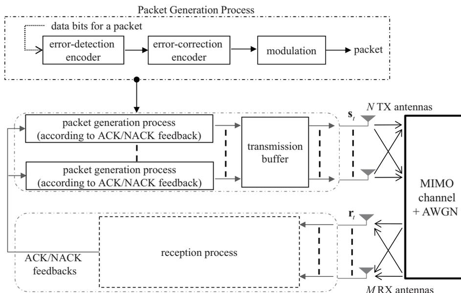
Figure 1. MMARQ system model block diagram.
