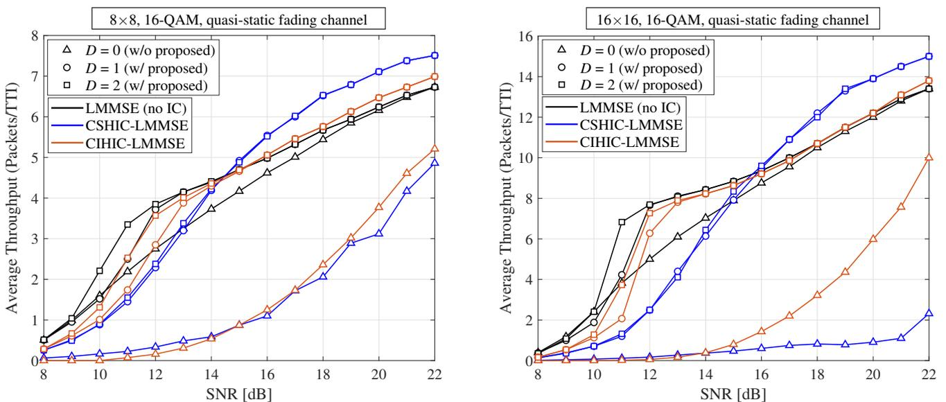
Figure 14. The average throughputs for  $8 \times 8$  and  $16 \times 16$  MMARQ systems with LMMSE and 16-QAM under the quasi-static fading channel.
