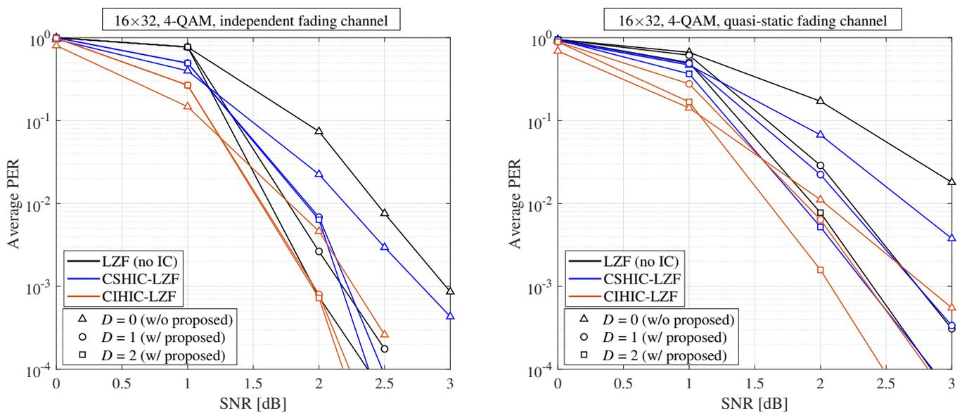
Figure 7. The average PERs for  $16 \times 32$  MMARQ systems with LZF and 4-QAM.
