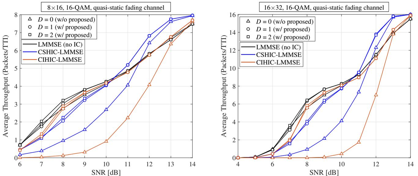
Figure 16. The average throughputs for  $8 \times 16$  and  $16 \times 32$  MMARQ systems with LMMSE and 16-QAM under the quasi-static fading channel.
