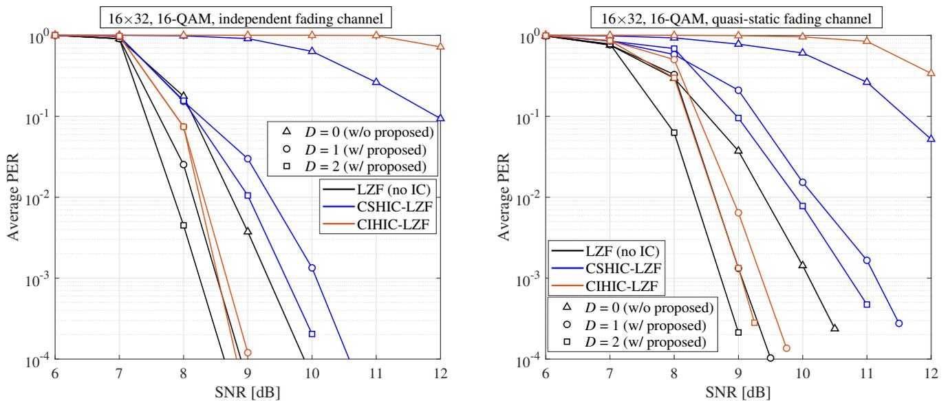
Figure 9. The average PERs for  $16 \times 32$  MMARQ systems with LZF and 16-QAM.
