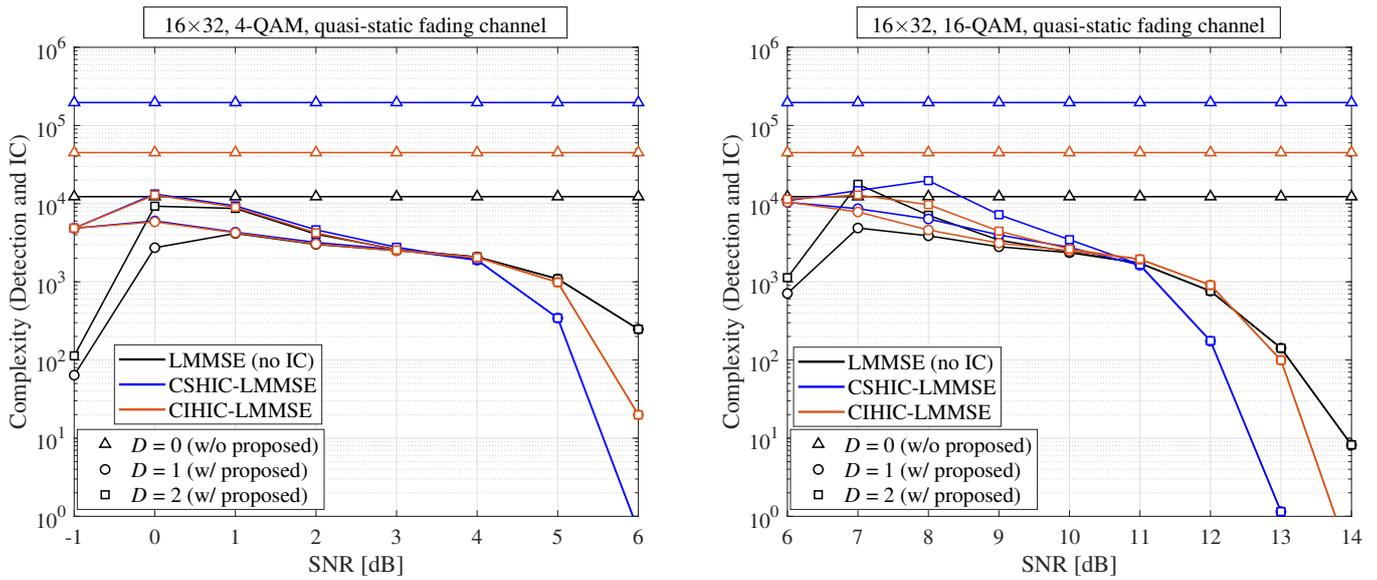
**Figure 17.** The complexity of detection per receive signal vector for  $16 \times 32$  MMARQ systems with LMMSE under the quasi-static fading channel.
