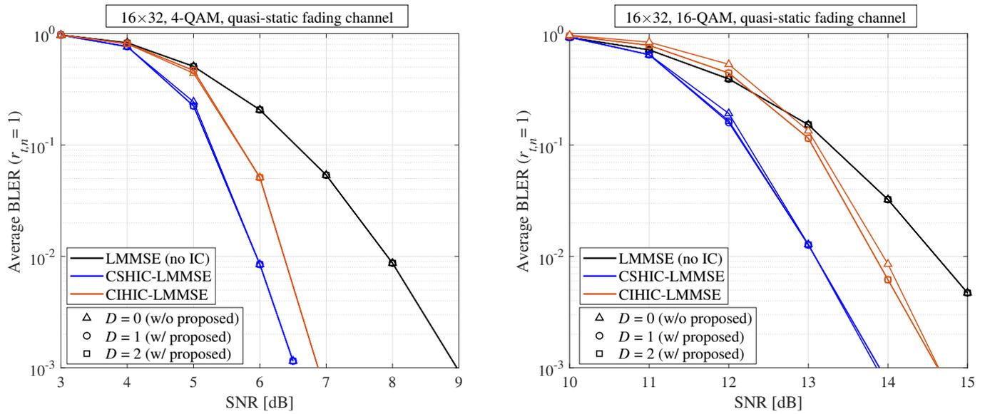
**Figure 10.** The average BLERs of 1st HARQ round for  $16 \times 32$  MMARQ systems with LMMSE under the quasi-static fading channel.
