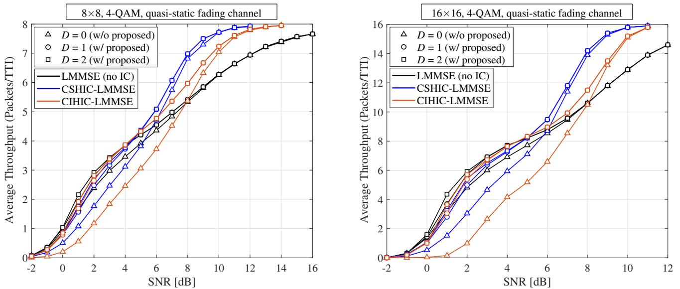
Figure 13. The average throughputs for  $8 \times 8$  and  $16 \times 16$  MMARQ systems with LMMSE and 4-QAM under the quasi-static fading channel.
