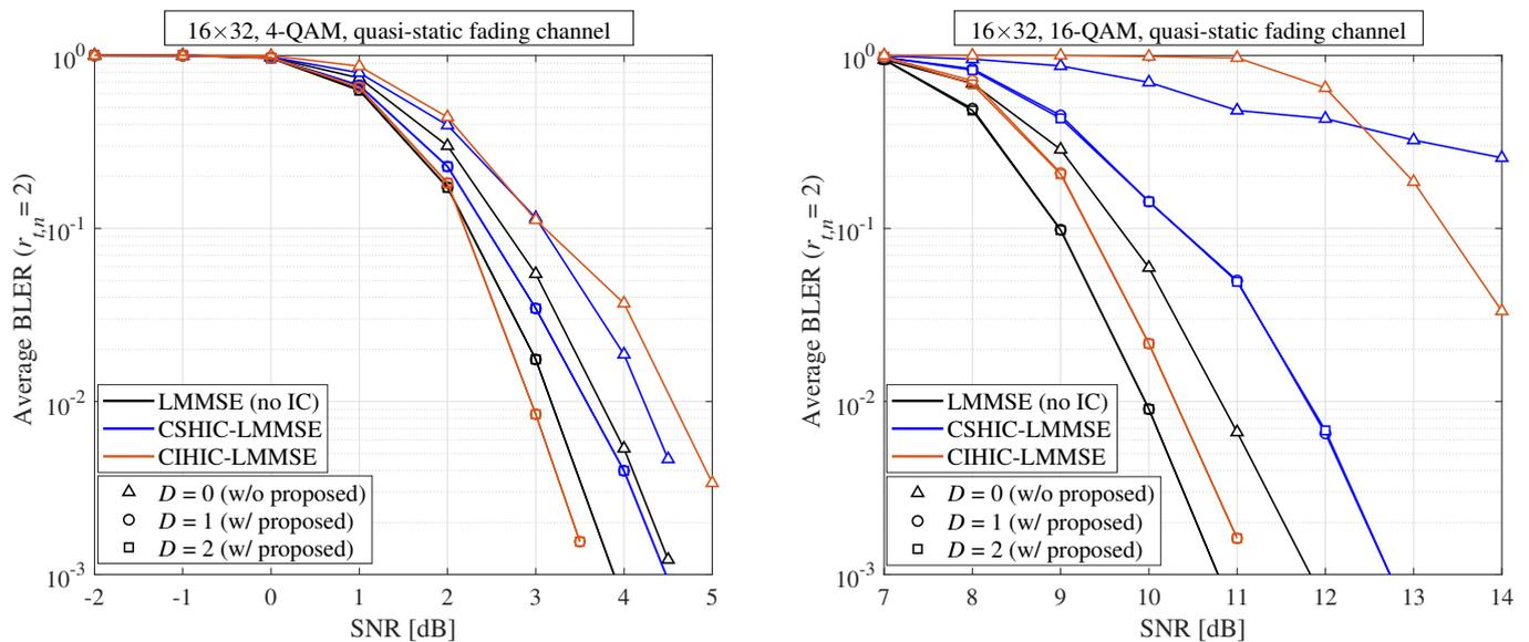
**Figure 11.** The average BLERs of 2nd HARQ round for  $16 \times 32$  MMARQ systems with LMMSE under the quasi-static fading channel.
