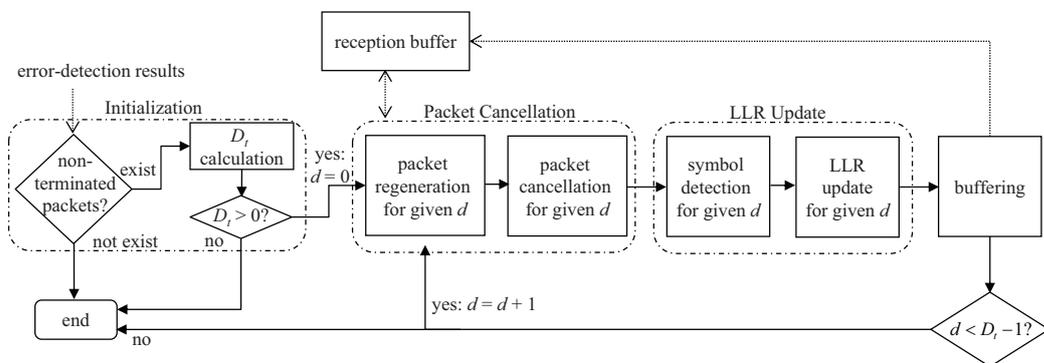
Figure 5. The block diagram of the proposed LLR refining scheme.
