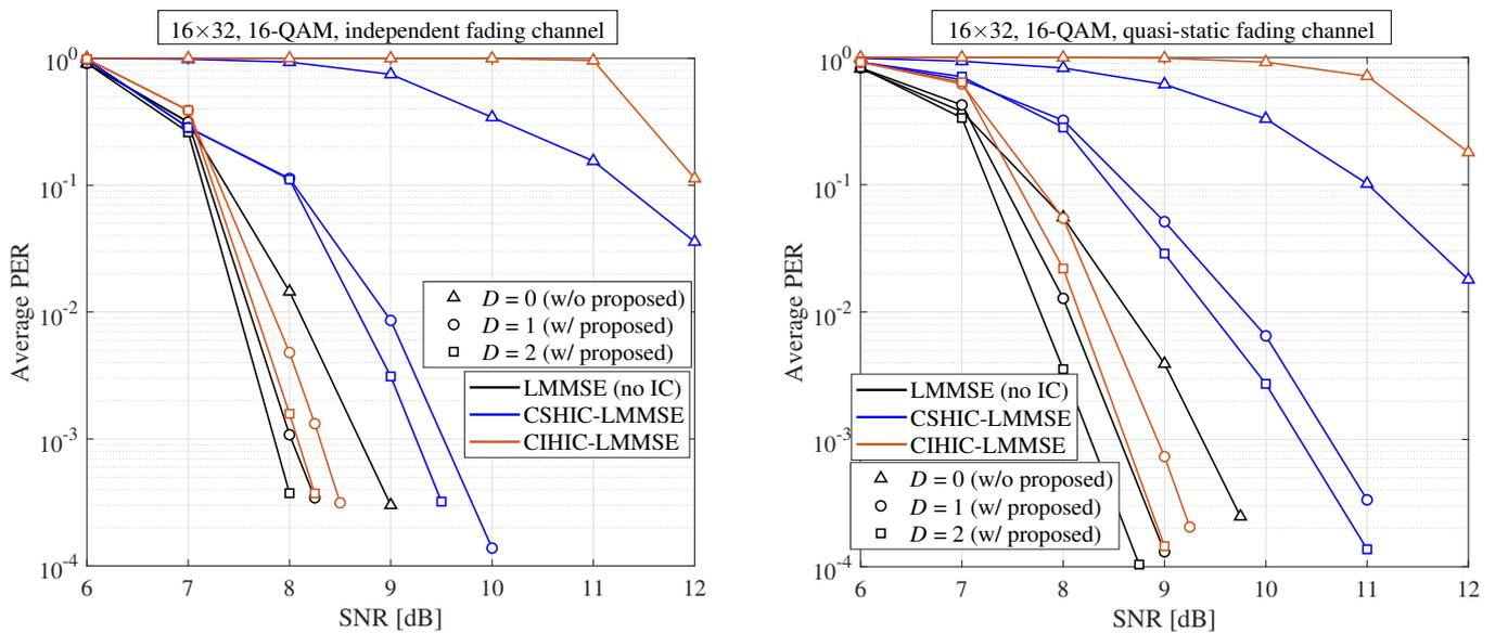
Figure 8. The average PERs for  $16 \times 32$  MMARQ systems with LMMSE and 16-QAM.
