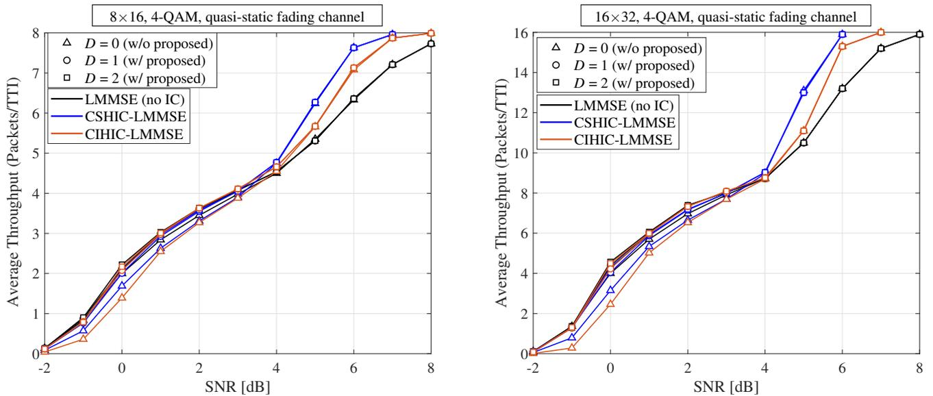
Figure 15. The average throughputs for  $8 \times 16$  and  $16 \times 32$  MMARQ systems with LMMSE and 4-QAM under the quasi-static fading channel.
