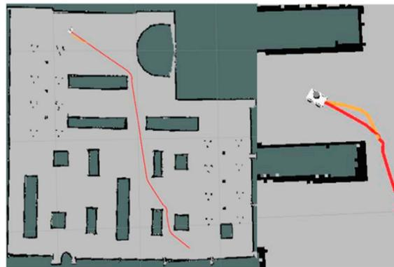
**Figure 10.** In the navigation experiment of the navigation system in Figure 4a, the red line segment represents the global path, while the yellow line segment represents the local path.
