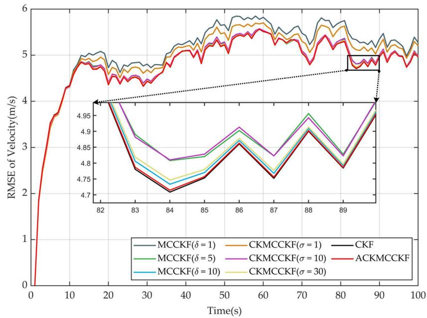
**Figure 3.** The velocity RMSE of each filtering algorithm under Gaussian measurement noise.
