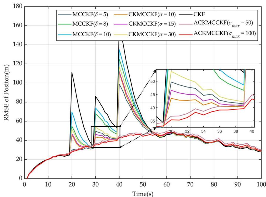
**Figure 7.** The position RMSE of each filtering algorithm under observation outliers.
