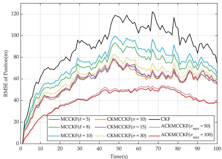
**Figure 4.** The position RMSE of each filtering algorithm under non-Gaussian measurement noise.
