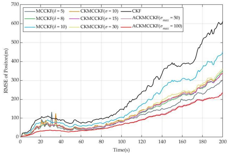
**Figure 6.** The position RMSE of each filtering algorithm in a 9-DoF system.
