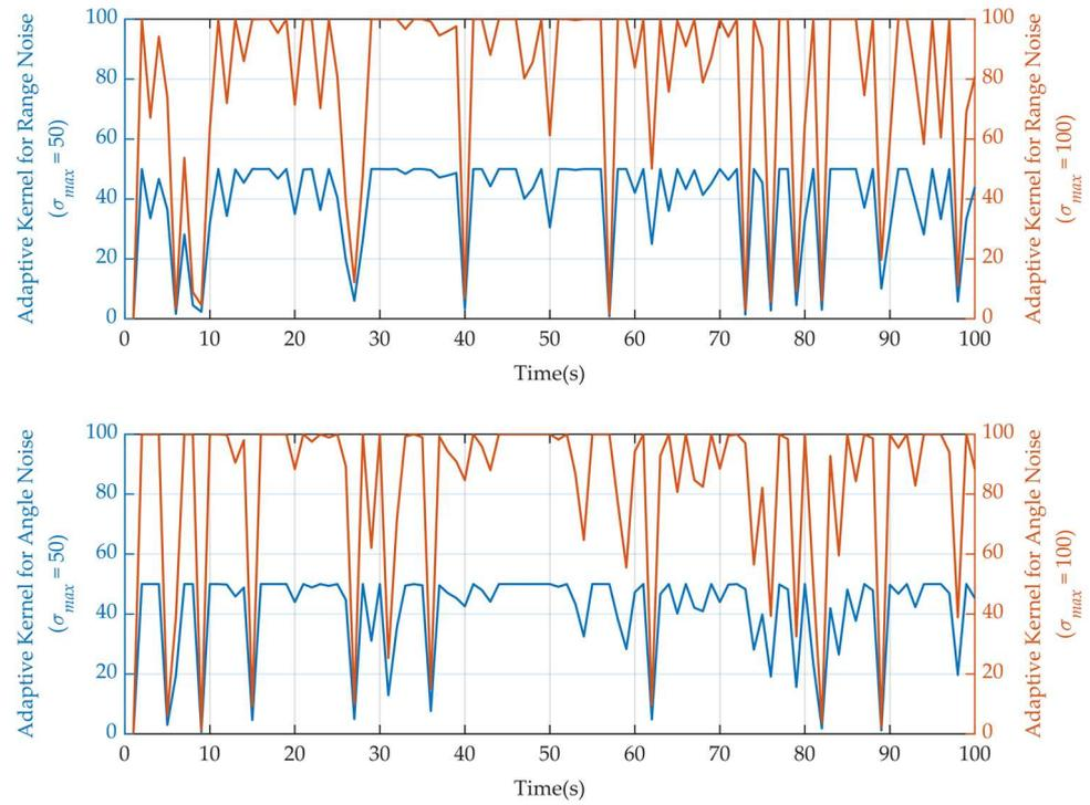
**Figure 5.** The adaptive kernel size of ACKMC-CKF with different kernel bandwidth upper limits in Experiment 2.
