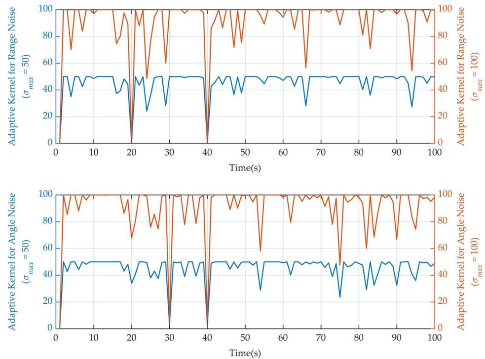
**Figure 8.** The adaptive kernel size of ACKMC-CKF with different kernel bandwidth upper limits in Experiment 3.
