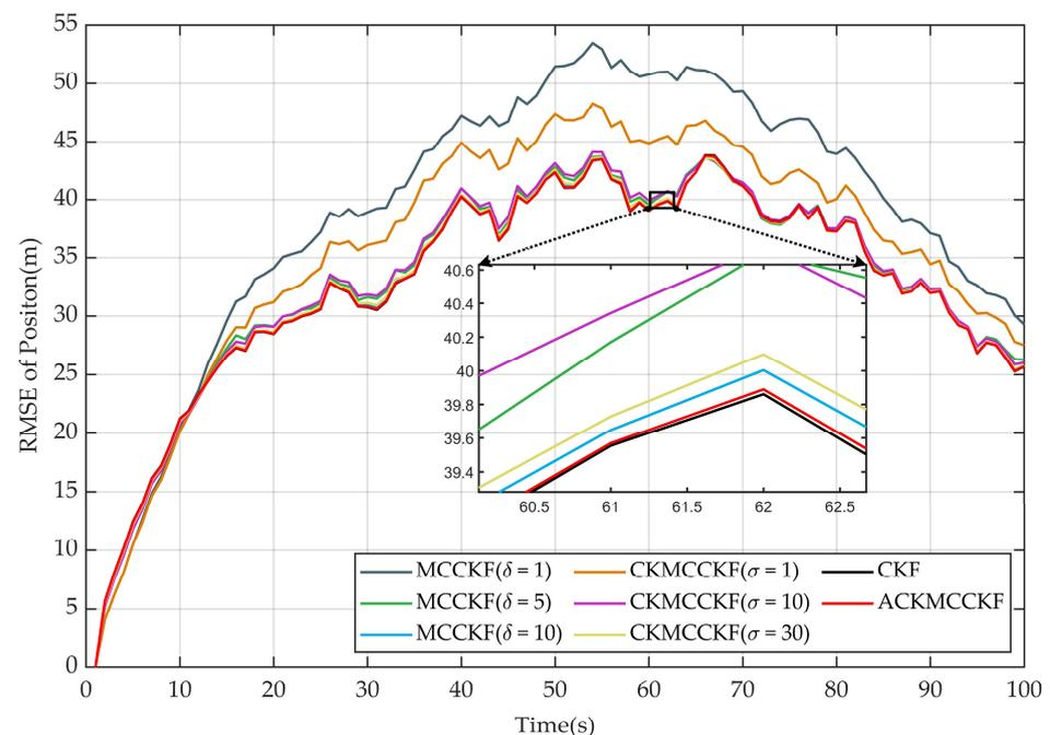
**Figure 2.** The position RMSE of each filtering algorithm under Gaussian measurement noise.
