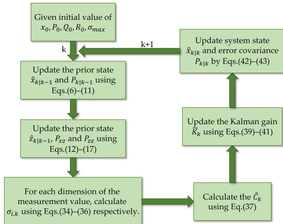
Figure 1. Flowchart of the proposed ACKMC-CKF algorithm.
