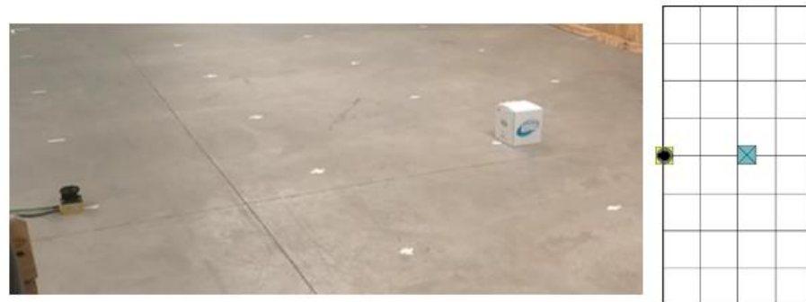
Figure 17. Position test, target at (0,2). The object is located in front of the LIDAR. The angle from the LIDAR to the object is 0^\circ . There are not any obstacles between the LIDAR and the object. The LIDAR is represented by a yellow square and the object by a blue one.
