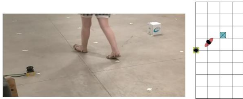
Figure 22. Crossing test, target remains in front of the lidar. The target is located at (-1,2) . An unexpected element crosses between the target and the LIDAR, and it is detected as a crossing object. The LIDAR is represented by a yellow square, the object by a blue one, and the person by a pink ellipse.
