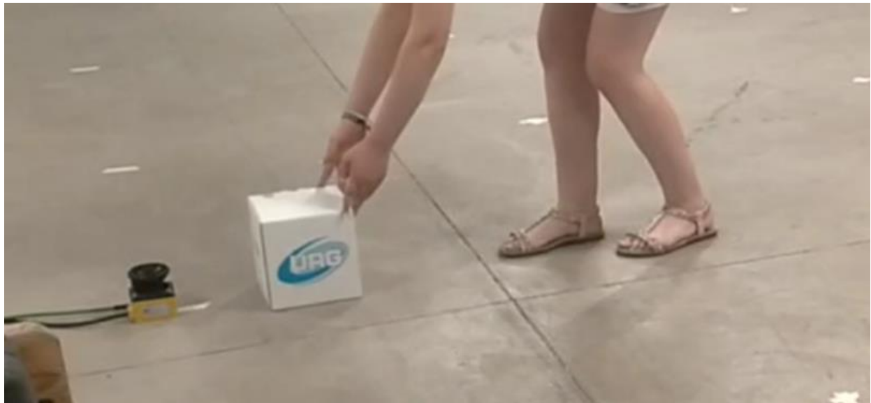
Figure 19. Position test, moving the target closer to the lidar. The object is placed very close to the LIDAR, so the velocity drops rapidly toward 0.
