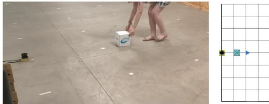
Figure 16. Position test, moving the target to (0,2). The object is moved carefully from (0,1) to (0,2), avoiding obstructing the LIDAR. The LIDAR is represented by a yellow square and the object by a blue one.
