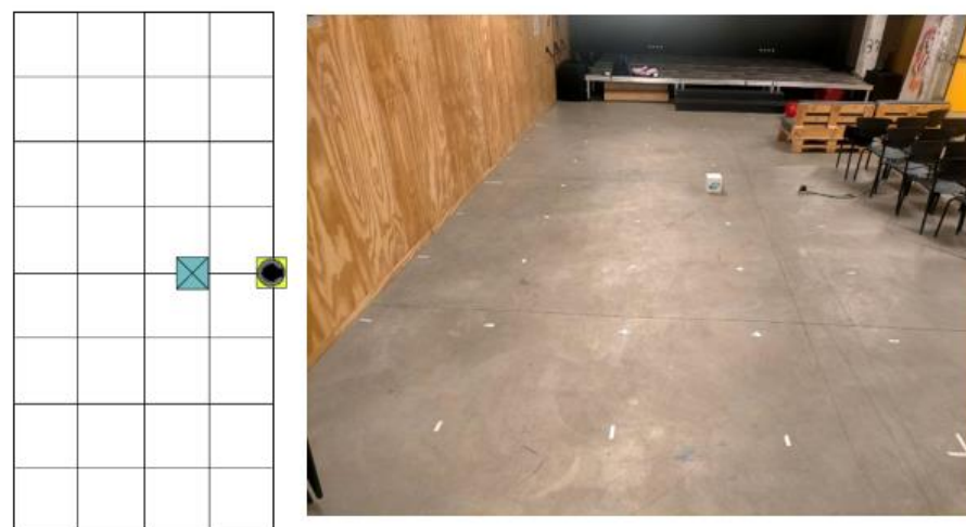
Figure 14. Static test environment setup. The LIDAR is in a static location, placed on the floor without the AGV. The object to be detected is the box of the LIDAR. The LIDAR is represented by a yellow square and the object by a blue one.
