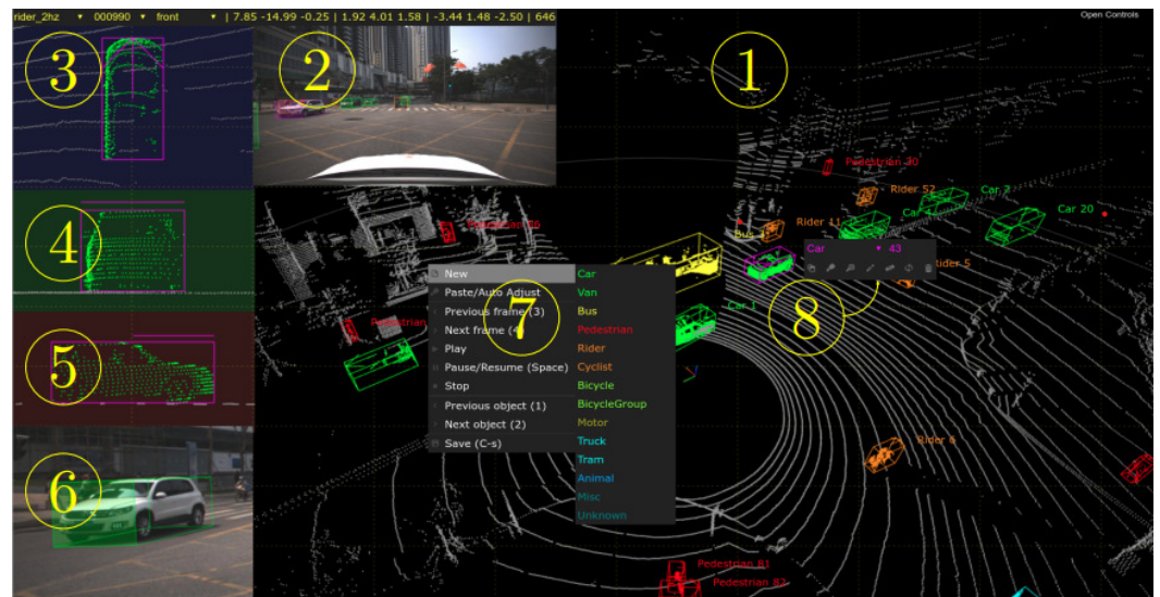
Figure 2. The main UI of SUSTechPoints. ① the perspective view of the 3D point cloud; ② the photo context, which is resizable and can be automatically switched among multiple camera images; ③ the top view of the selected object; ④ the front view of the selected object; ⑤ the side view of the selected object; ⑥ the focused photo context, which can be automatically chosen for the selected object; ⑦ the context menu, which provides tools of context operations; ⑧ the floating fast toolbox, which provides most used tools.
