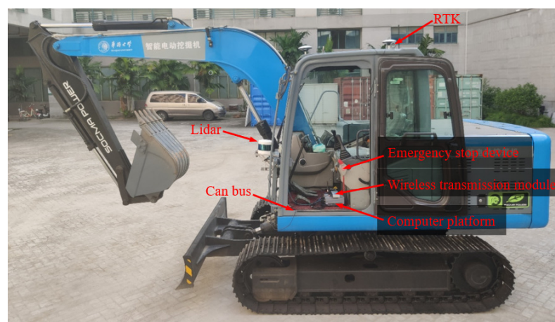
Figure 22. Tracked construction machinery real vehicle test platform.
