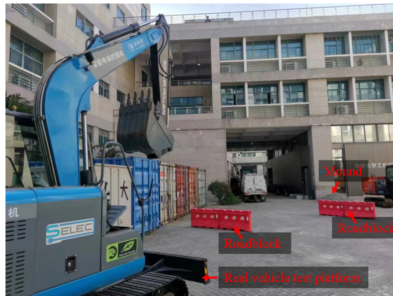
Figure 24. Autonomous path finding and obstacle avoidance test scenario of real vehicle.
