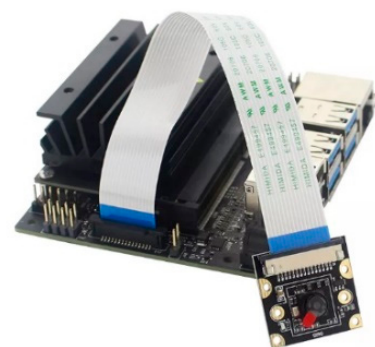
Figure 24. Jetson nano-powered mobile robot with 8-megapixel Raspberry Pi camera module.
