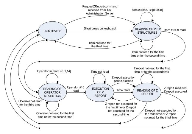
Figure 10. A state diagram of the complete Z report workflow.
