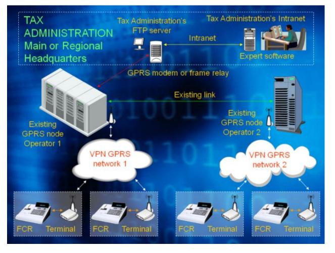
Figure 5. The subsystem for remote control of fiscal cash registers.
