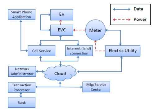
Figure 2. The subsystem for remote control of EV chargers.
