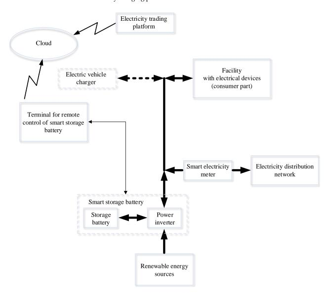
Figure 3. The subsystem for remote control of smart batteries.
