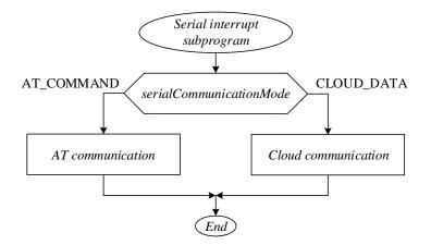
Figure 9. Serial interrupt subprogram.
