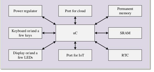
Figure 6. Block schematic of the hardware for the terminal.
