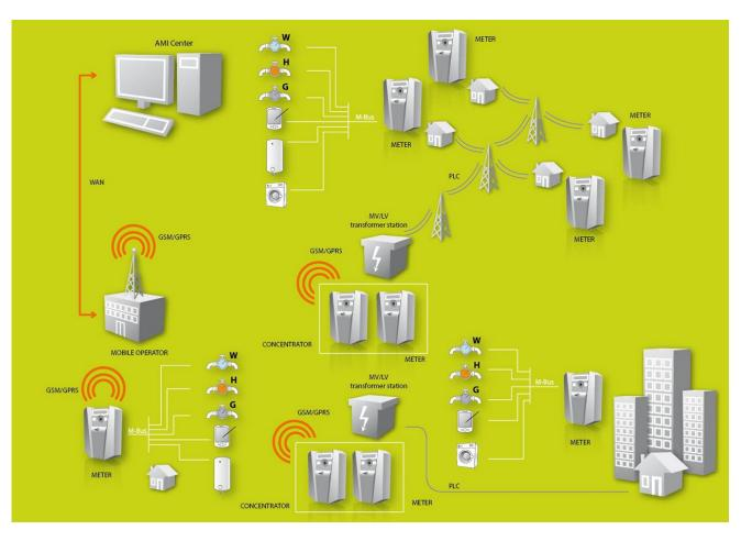
Figure 4. The subsystem for remote control of smart meters.
