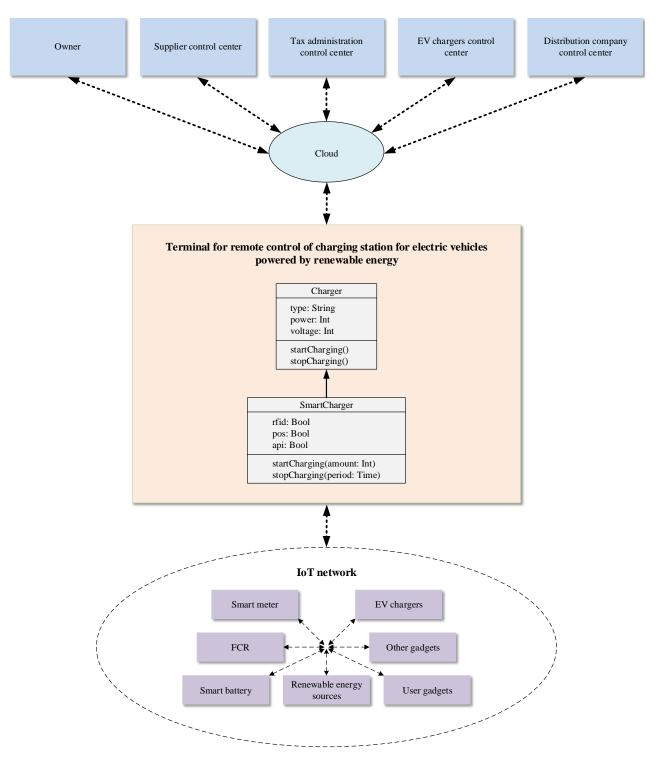
**Figure 1.** Block schematic of the design of the system for remote control of charging station for electric vehicles powered by renewable energy.
