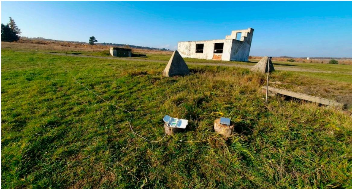
**Figure 13.** Installation of the polarization sensor and supply cabling in the Březina military area.
