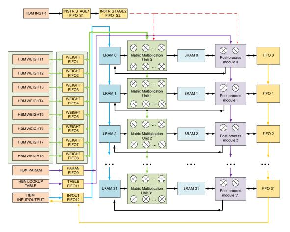
Figure 3. The architecture of the kernel (LSTM accelerator running on PL).
