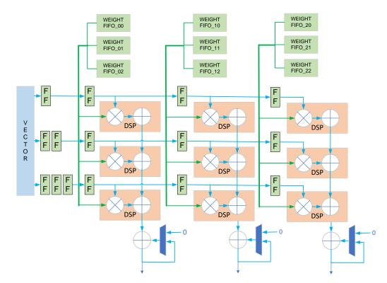
Figure 4. Design of matrix multiplication unit.
