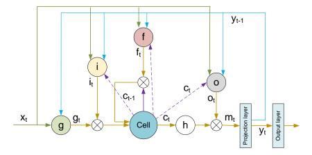
Figure 1. LSTM network structure.
