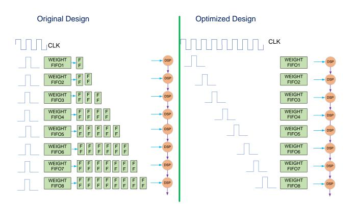
Figure 5. Optimized data read timing.
