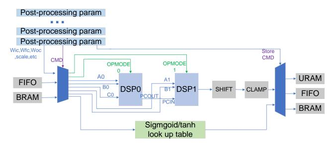
Figure 6. Structure of the post-processing unit.
