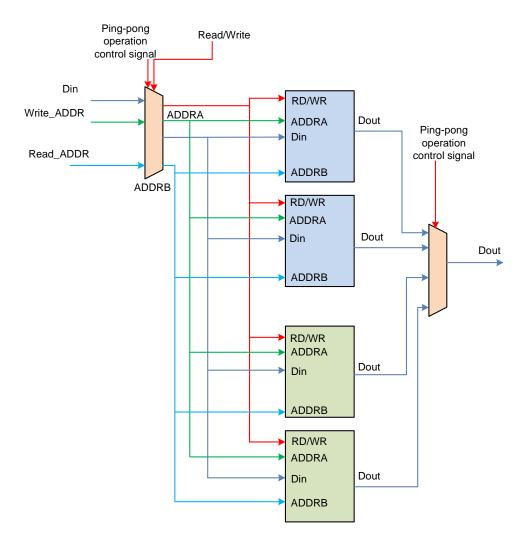
Figure 7. Structural diagram of the double buffer.
