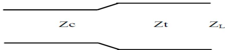
Figure 4. Adaptation by quarter-wave transformer.
