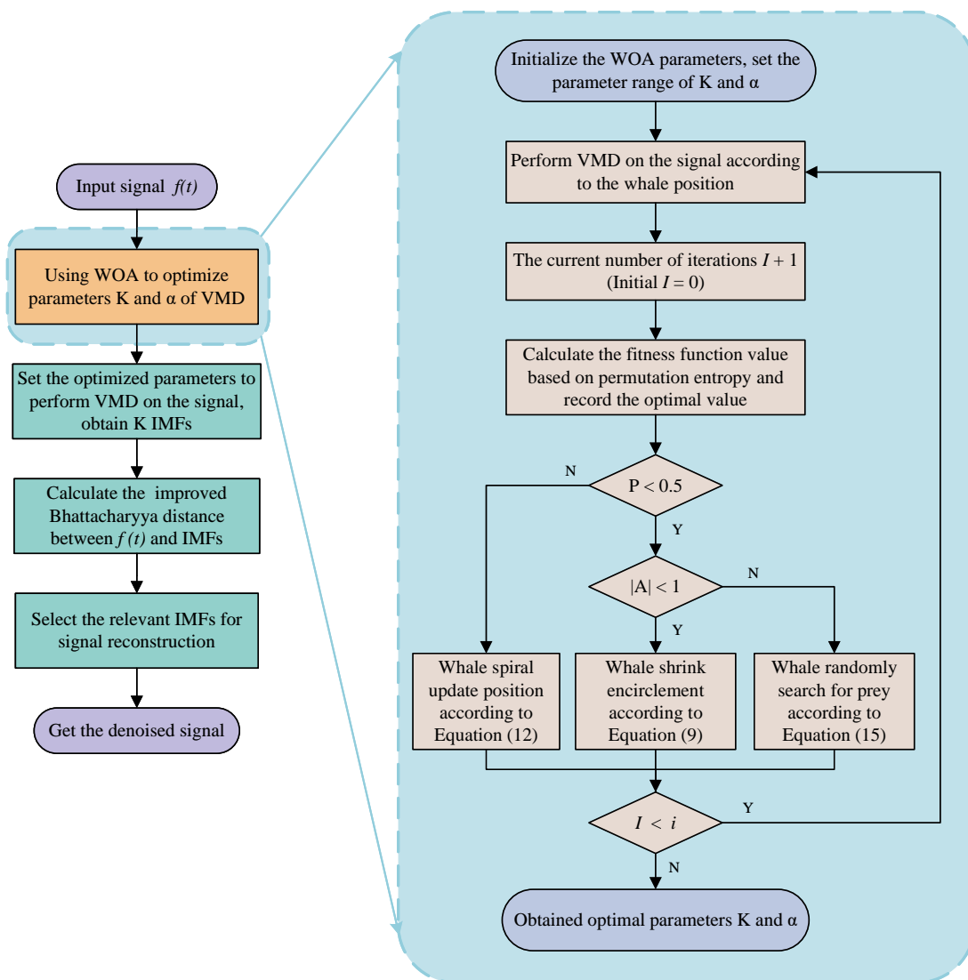
Figure 1. Flow chart of signal denoising method based on WOA-VMD-BD.
