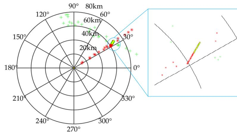
**Figure 9.** True target fusion results with a jamming range delay of 0 km including overall rendering and partly enlarged view, where green line (plus) denotes the track detected by radar 1, red line (asterisk) is detected by radar 3, and yellow line (dotted) is the target track that satisfies the fusion criterion.
