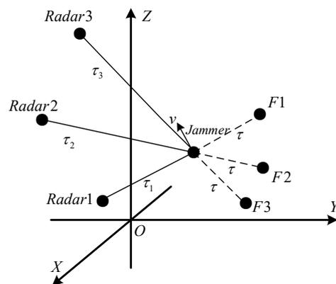
Figure 2. Geometric position distribution of three radars and a jammer.
