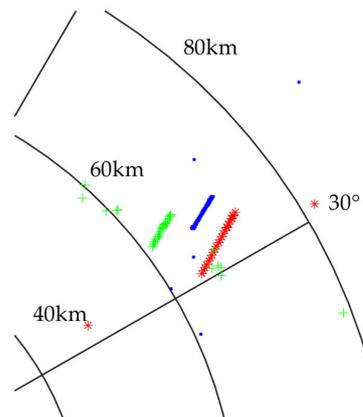
**Figure 7.** Three tracks in the radar 3 coordinate system, where green line (plus) is detected by radar 1, blue line (dotted) is detected by radar 2, and red line (asterisk) is detected by radar 3.
