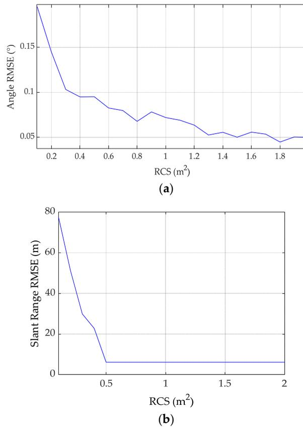
**Figure 8.** Target angle and slant range error estimation results: (a) RMSE of angle versus target RCS; (b) RMSE of slant range versus target RCS.
