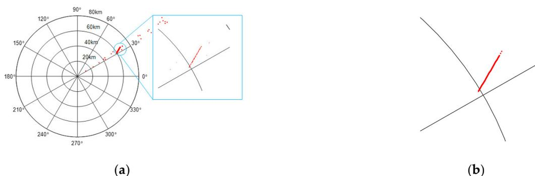
Figure 5. The moving target track detected by ground-based radar in polar coordinates: (a) before interpolation; (b) after interpolation.
