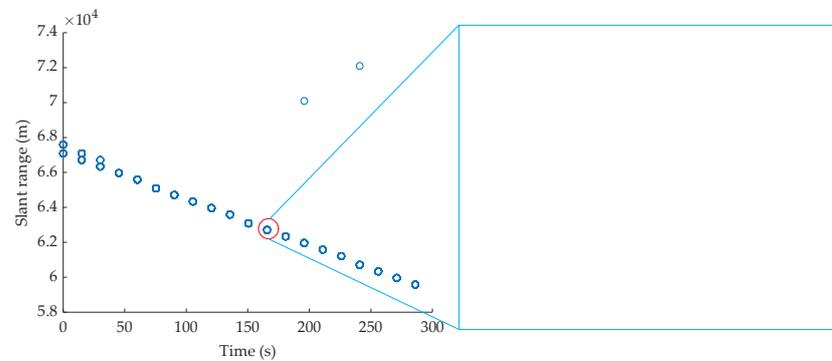
Figure 4. The range transformation of jamming with an enlarged view of radar main-lobe pulse sequence in a circle.
