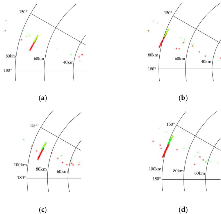
**Figure 10.** Fusion performance analysis in a two-radar system: (a) Target track fusion results when the jamming range delay is set as 10 km; (b) target track fusion results when the jamming range delay is set as 20 km; (c) jamming range delay is 30 km; (d) jamming range delay is 40 km (green line (plus) is detected by radar 1, red line (asterisk) is detected by radar 3, yellow line (dotted) is track that satisfies fusion criterion).
