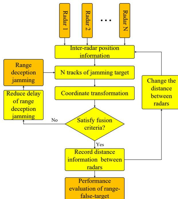
Figure 6. Flowchart for the jamming performance evaluation.
