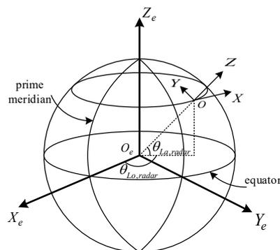
Figure 3. Earth-fixed coordinate system and radar local coordinate system.
