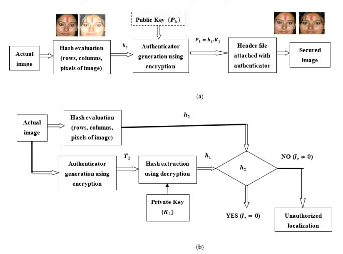
**Figure 5.** System for image authentication using cryptography following public & private key; (a) authenticator generator; (b) authenticity verification.
