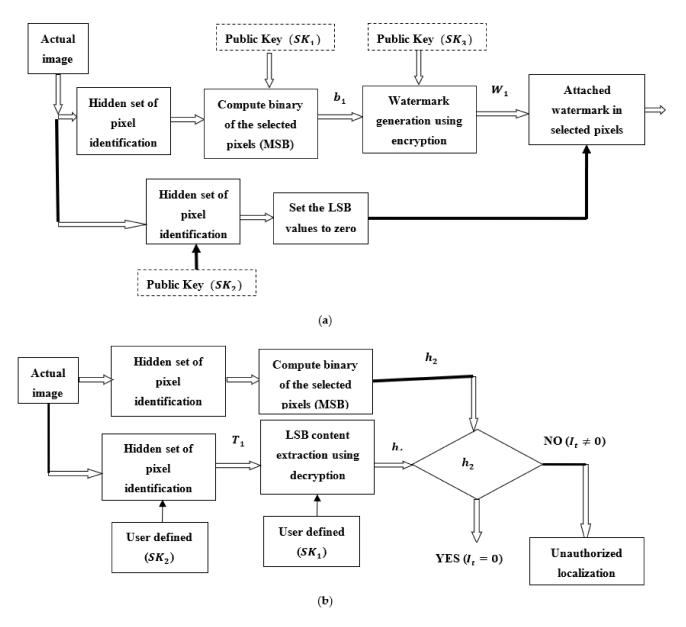
**Figure 6.** Image authentication using robust watermarking; (**a**) verifier generator; (**b**) authenticity confirmation.
