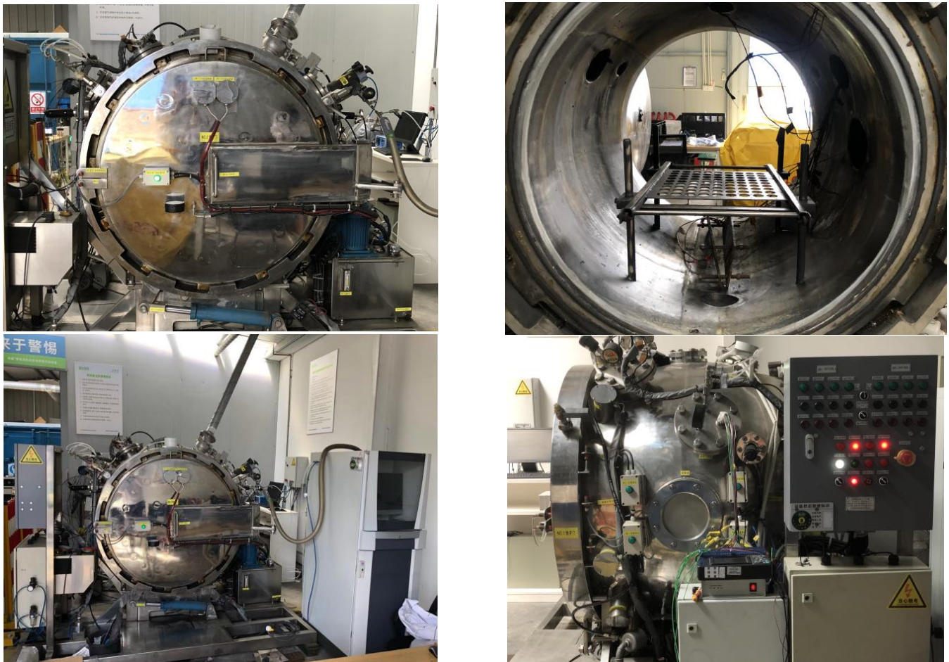
Figure 1. Physical picture of AEC constant volume adiabatic explosion chamber.
