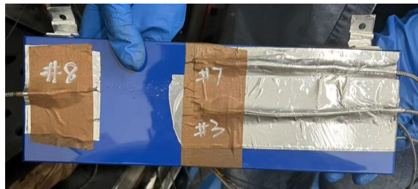
Figure 3. Thermocouple paste method diagram.
