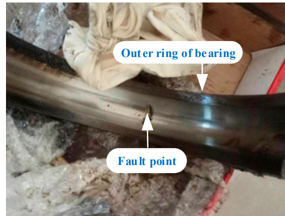
Figure 6. Outer ring fault of rolling bearing at driving end of wind power generator.
