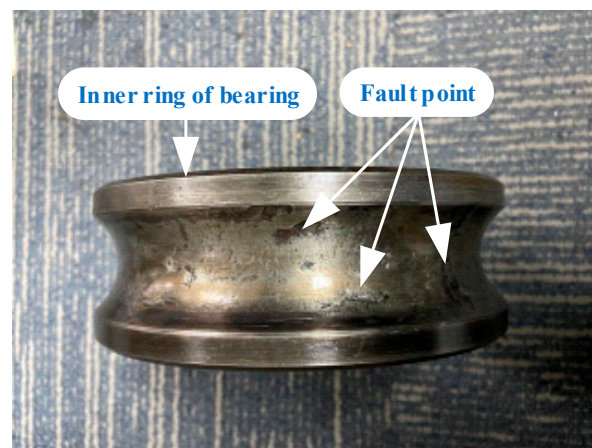
Figure 10. The inner ring fault of rolling bearing at driving end of wind power generator.
