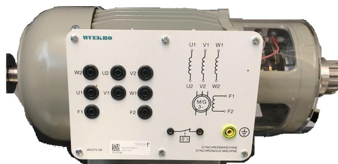
Figure 7. WUEKRO Wound Rotor Separated Excited Synchronous Motor (WRSESM).
