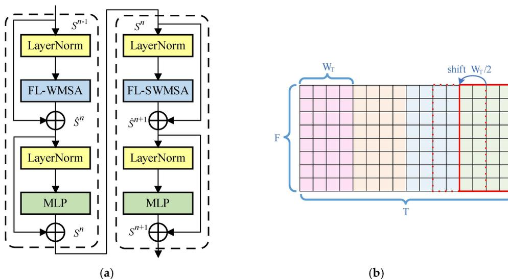
**Figure 3.** (a) The structure of a frame-level Swin Transformer layer. (b) The illustration of the window self-attention mechanism of a frame-level Swin Transformer.
