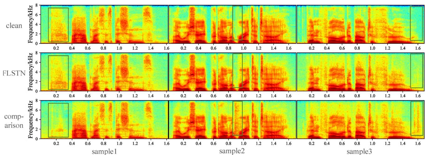
**Figure 6.** Enhanced spectrograms of FLSTN and comparison model (samples are saved at 16 KHz).
