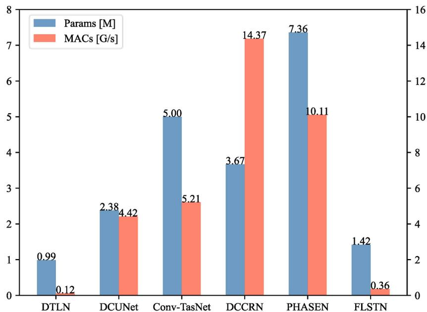
**Figure 5.** Complexity comparison with various competing network models.
