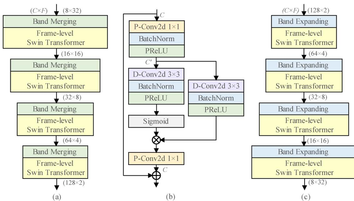
Figure 2. (a) The detail of encoder. (b) The proposed lightweight TFCM. (c) The detail of decoder.
