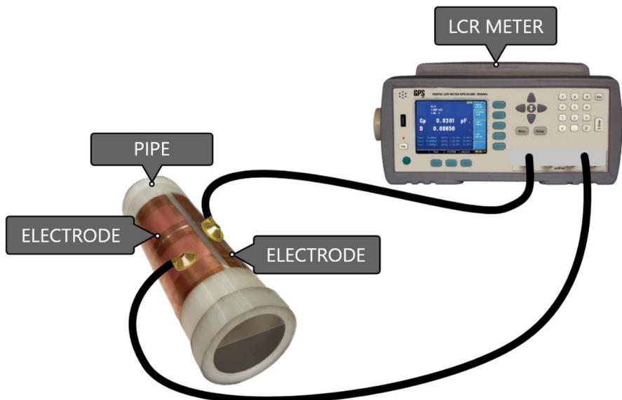
**Figure 3.** Measuring the capacitance value of pipe with a horizontal concave sensor using an LCR meter.
