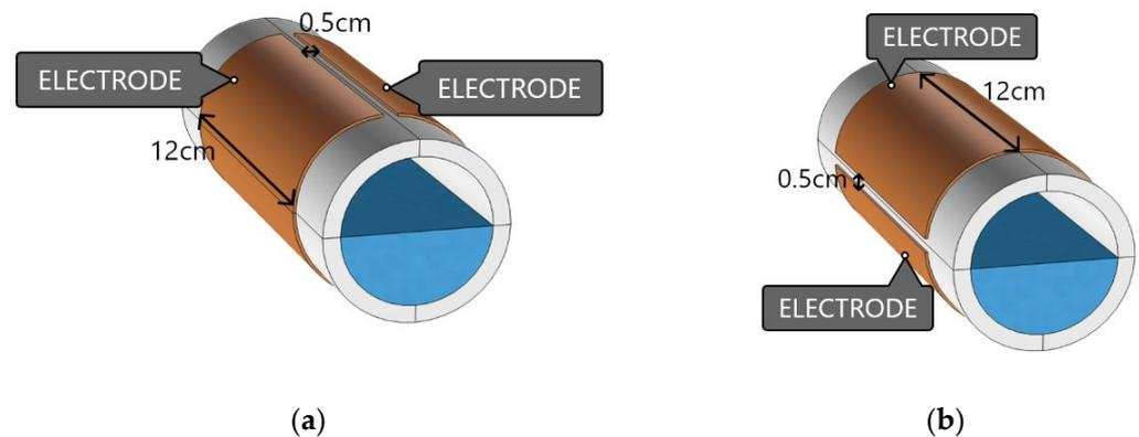
**Figure 4.** Diagram of a concave sensor for two-phase stratified flow, (a) Horizontal orientation, (b) Vertical orientation.**Table 2.** Measured capacitance values at different void fractions for the concave sensor.
