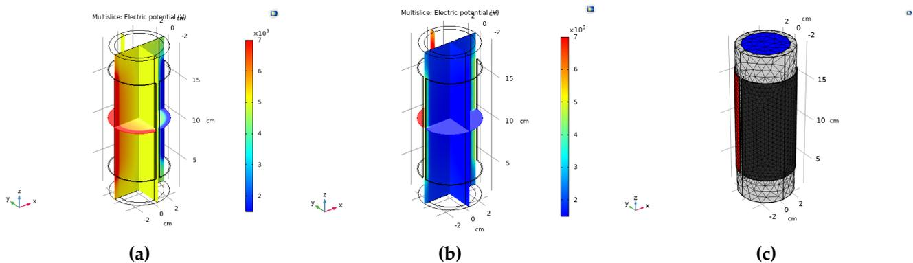
Figure 9. Electrical potential of the concave sensor in (a) Horizontal orientation, (b) Vertical orientation and (c) Meshed model of the horizontal concave sensor.
