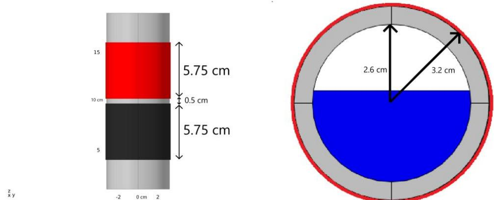
**Figure 7.** Dimensions of the double-ring designed by COMSOL simulation where the blue color represents the water level, the gray color represents the pipe, and the red and black colors represent the electrodes.
