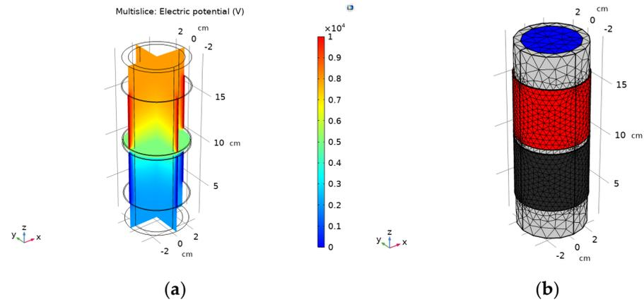
**Figure 6.** Double-ring sensor in stratified two-phase flow simulation (a) schematic of electric potential where red color represents high potential and blue color represents low potential, (b) meshed model.
