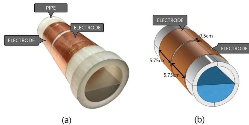
**Figure 2.** Double-ring sensor, (a) Experimental, (b) Simulation where the blue color represents the water level, the gray color represents the pipe, and the red color represents the electrodes.
