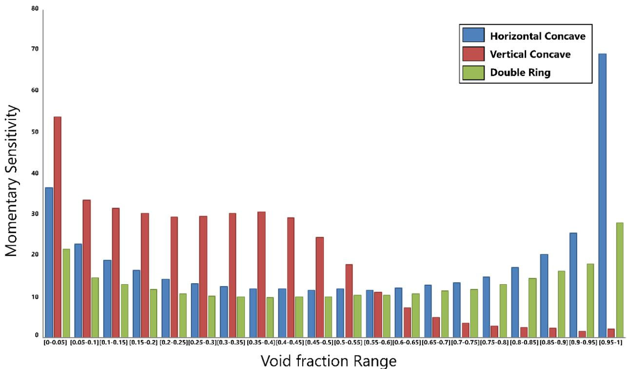
Figure 11. Comparing horizontal concave, vertical concave, and double-ring sensors in different ranges.
