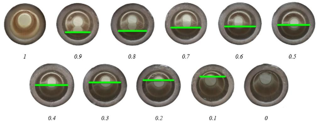
**Figure 1.** Different water levels in the cross-section of the pipe to create different void fractions in the experimental experiment where the water level is highlighted with a green line on each image of different void fractions.
