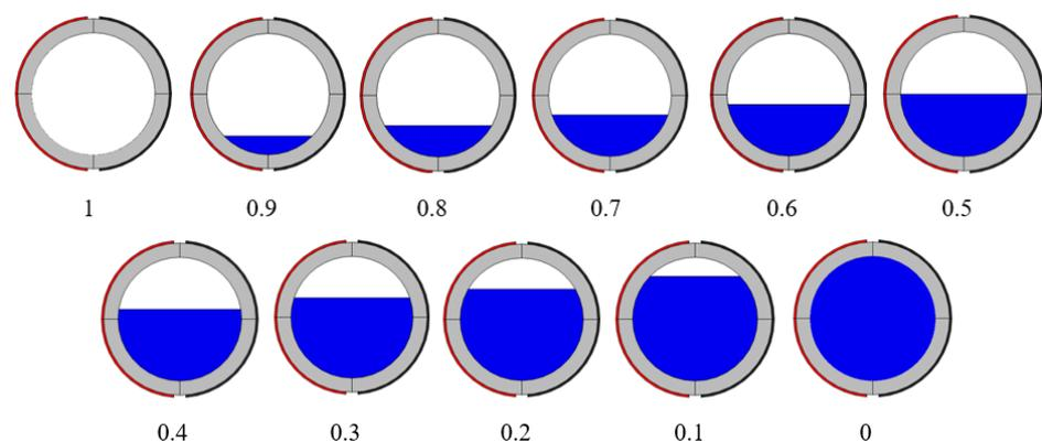
**Figure 5.** Different water levels in the cross-section of the pipe for a different void fraction in COMSOL, where the blue color represents the water level, the gray color represents the pipe, and the red and black colors represent the electrodes.
