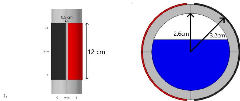
Figure 8. Simulated concave sensor along with its dimensions with the stratified two-phase flow where the blue color represents water level, the gray color represents the of the pipe, and the red and black colors represent the electrodes.
