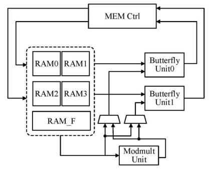
Figure 3. H-NTT module hardware architecture.
