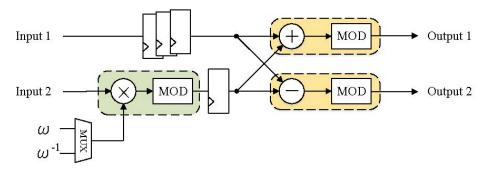
Figure 4. Butterfly unit hardware architecture.
