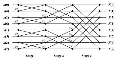
Figure 1. Eight-point DIT-NTT data flow diagram.
