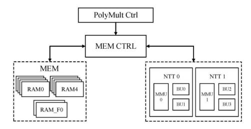
Figure 7. Polynomial multiplier overall architecture.
