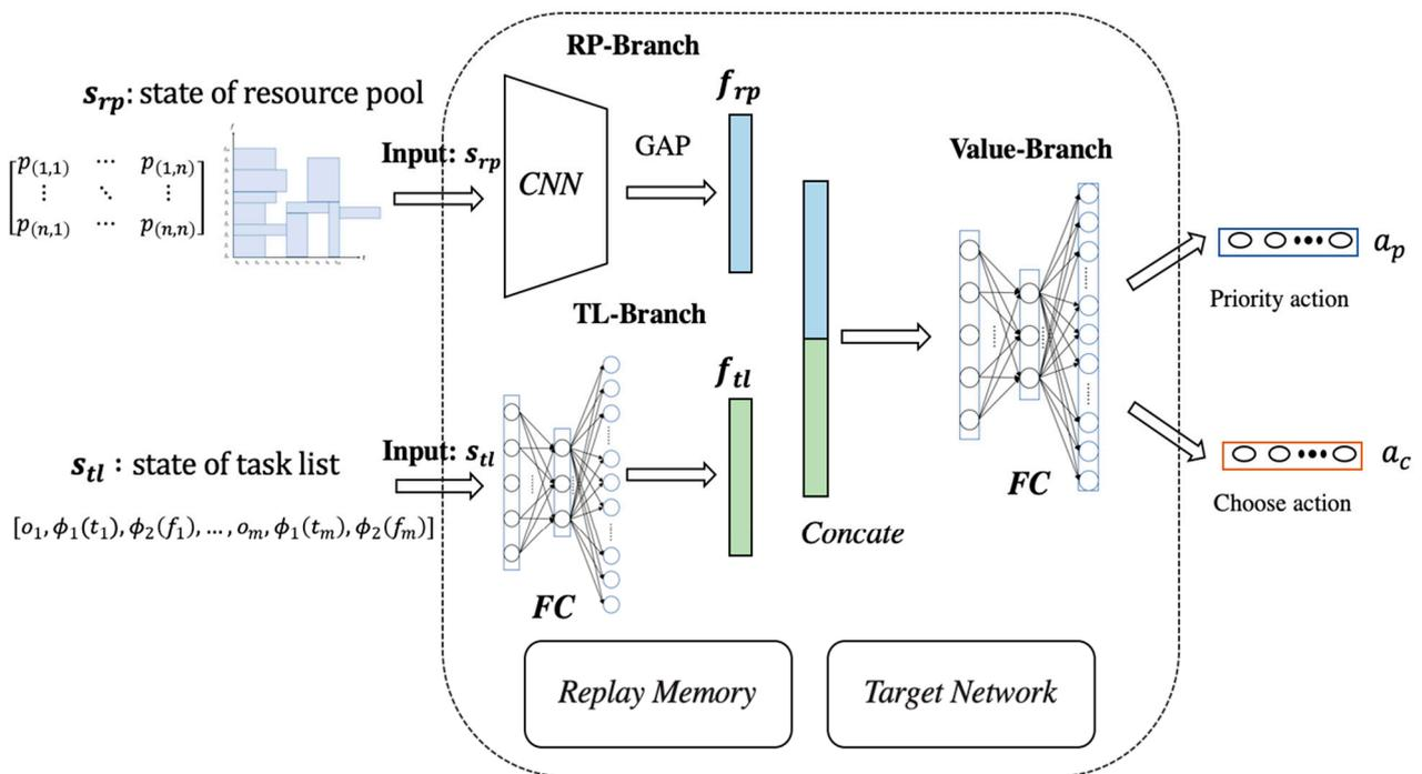
**Figure 4.** The structure of the proposed MBDQN resource allocation model.
