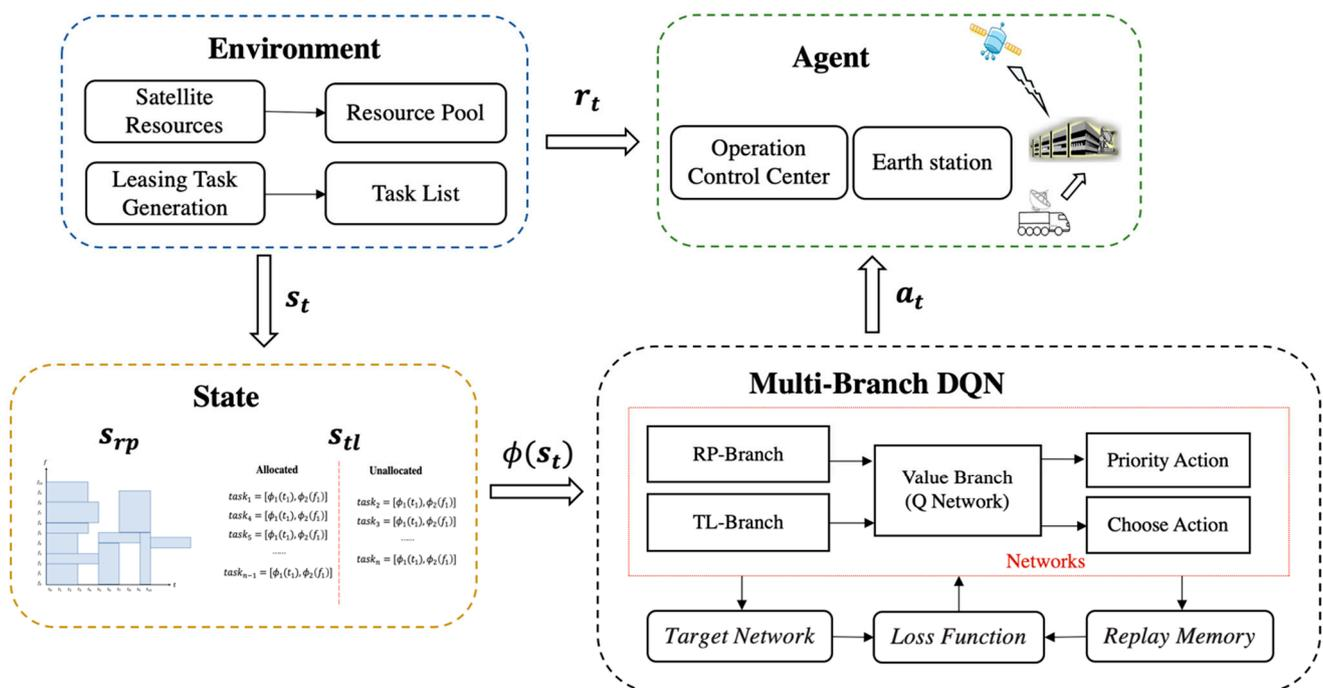
Figure 3. Overview of the proposed Multi-Branch DQN-based resource allocation method.
