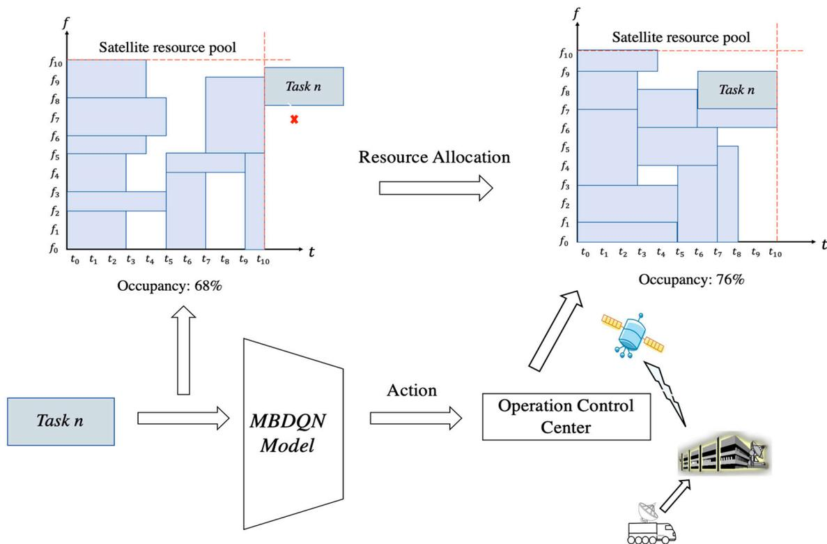
Figure 2. MBDQN is used to conduct efficient satellite resource allocation and improve resource occupancy.
