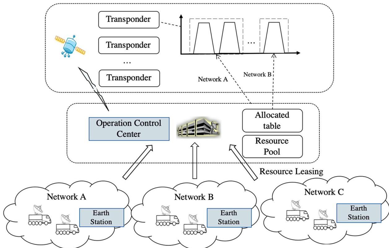
**Figure 1.** The process of transparent satellite transponder resource allocation.
