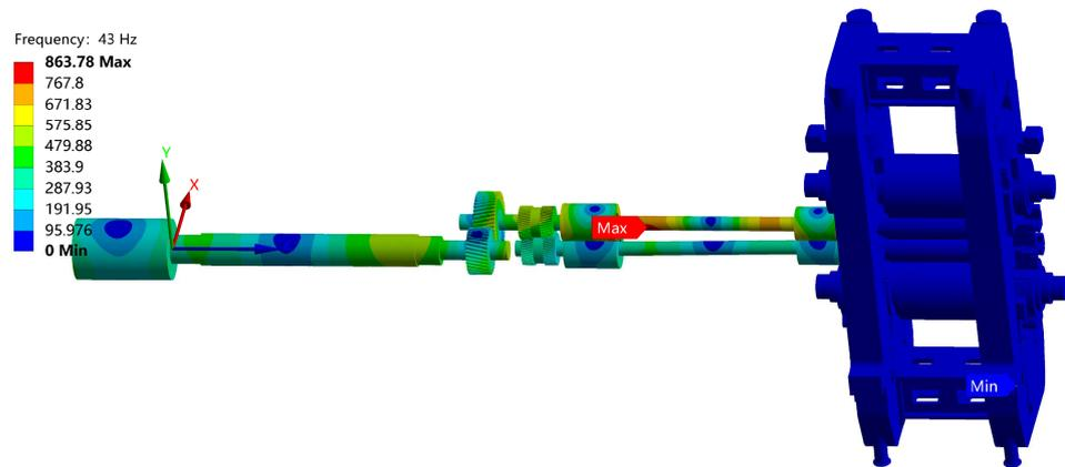
Figure 7. Harmonic response cloud for vibration energy flow of 43 Hz.
