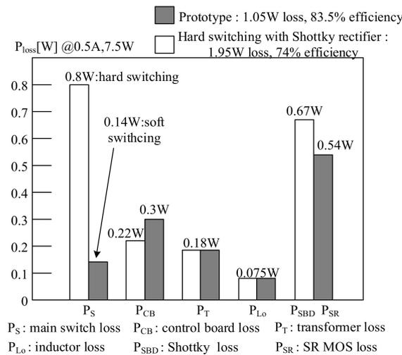
**Figure 8.** Estimated power loss comparison between the prototype and the traditional forward converter at 0.5 A load and 28 V input.
