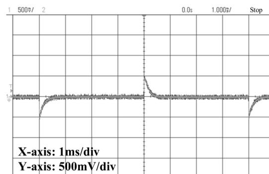
**Figure 12.** The output voltage waveform under load-step transient from 0.5 A to half load.
