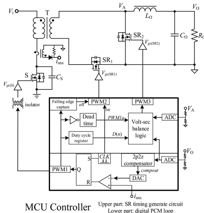
Figure 4. The proposed control diagram in DCM.
