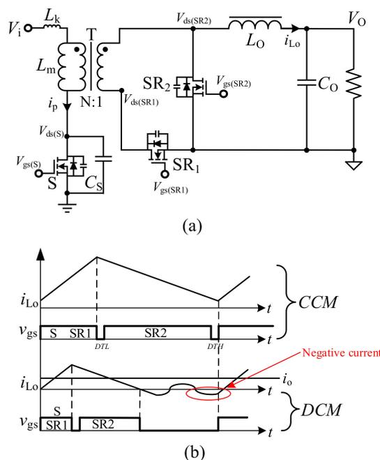
**Figure 1.** (a) Forward circuit with synchronous rectifiers. and (b) inductor current and gate-drive signal in continuous conduction mode and discontinuous conduction mode.
