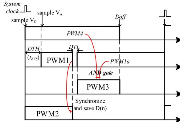
Figure 7. The waveform and generation of PWM signals.
