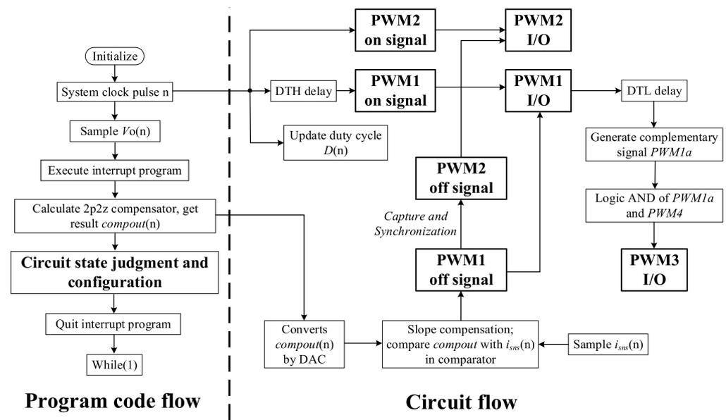
Figure 5. The control flow chart in DCM.
