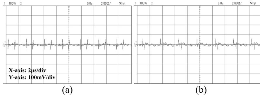
Figure 13. The output voltage ripple under (a) 0.5 A load and (b) full load.
