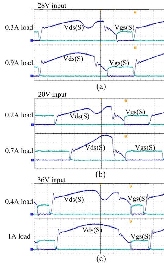
**Figure 11.** Drain-source voltage and gate-driver voltage of the primary switch at (a) 28 V input; (b) 20 V input; and (c) 36 V input. (X-axis: 400 ns/div; Y-axis:  $V_{ds(S)}$ : 20 V/div;  $V_{gs(S)}$ : 10 V/div). The small symbol “T” is the zero position of the time axis.
