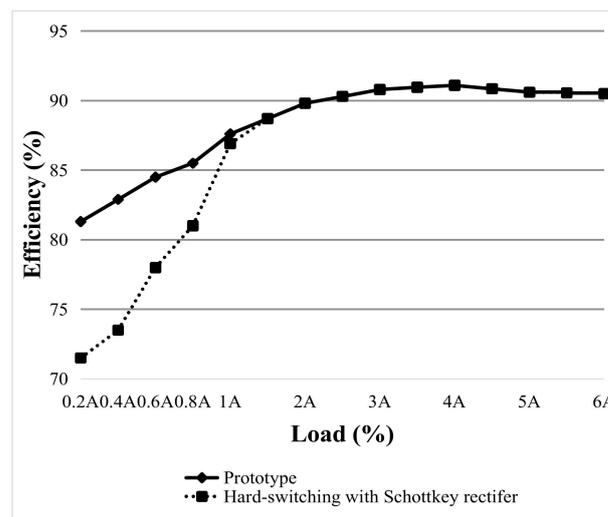
Figure 14. Efficiency comparison between the prototype and traditional forward converter at 28 V input.
