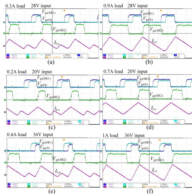
Figure 10. Gate-drive signal  $V_{gs(S)}$ ,  $V_{gs(SR1)}$ , and  $V_{gs(SR2)}$ ; inductor current waveforms  $I_{Lo}$  at (a) 28 V input, 0.3 A load; (b) 28 V input, 0.9 A load; (c) 20 V input, 0.2 A load; (d) 20 V input, 0.7 A load; (e) 36 V input, 0.4 A load; (f) 36 V input, 1 A load. (X-axis: 800 ns/div; Y-axis:  $V_{gs(S)}/V_{gs(SR1)}/V_{gs(SR2)}$ : 10 V/div,  $I_{Lo}$ : 1 A/div). The small symbol “T” is the zero position of the time axis.
