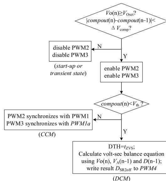
Figure 6. The workflow of circuit state judgement and configuration.
