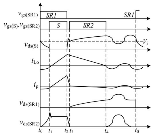
Figure 2. Key voltage and current waveforms of the proposed circuit.
