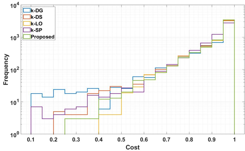
Figure 2. Histogram plot of the attackers' costs of launching DDoS Attack on an LEO satellite network.
