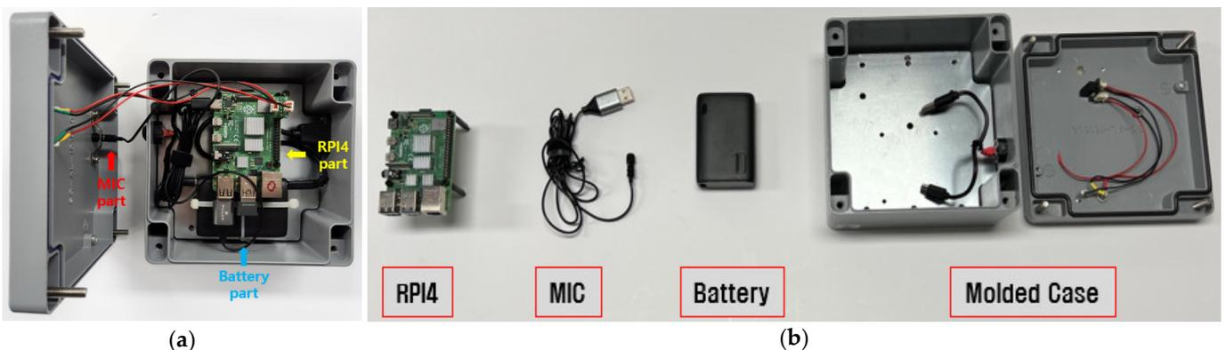
Figure 11. Internal structure of embedded system devices as: (a) embedded system internal structure; (b) embedded system internal equipment.
