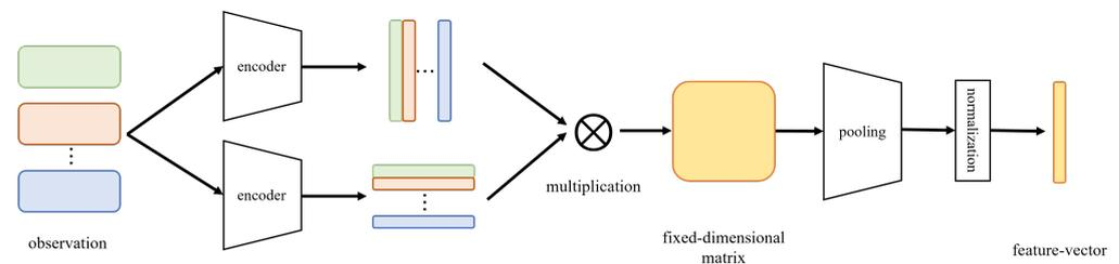
Figure 1. Data flow diagram of the variable-dimensional observation processing network.
