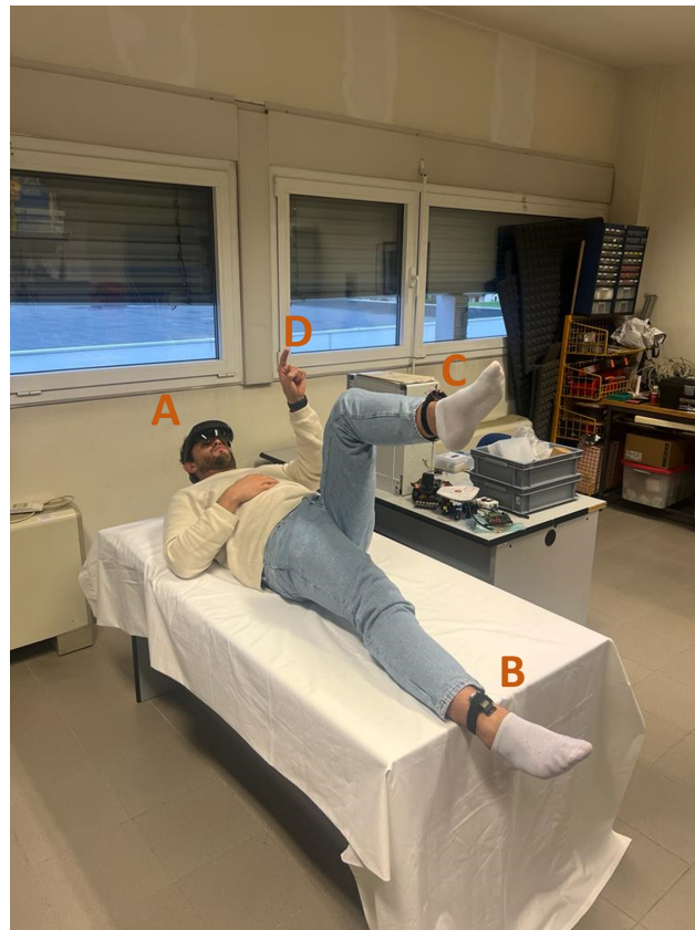
Figure 7. The experimental setup. (A) the AR headset; (B) the EmotiBit on the right leg; (C) our custom wearable IMU platform on the left leg; (D) the user interacting with the holograms while performing the exercise.
