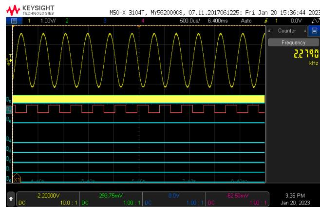
**Figure A1.** Lower frequency 2279 Hz generated waveform.
