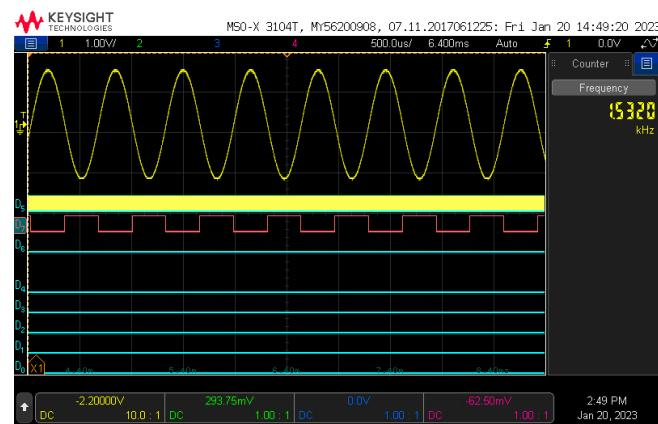
**Figure A7.** Lower frequency 1532 Hz generated waveform.
