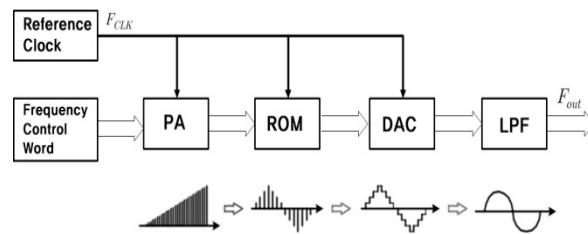
**Figure 8.** Basic structure of the proposed system.
