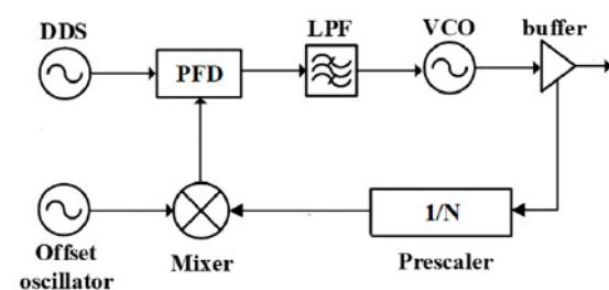
**Figure 7.** DDS-PLL block diagram.
