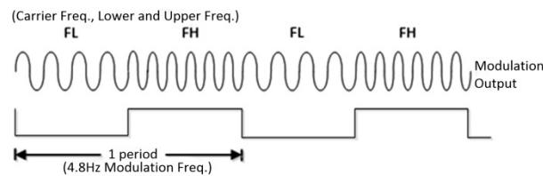
**Figure 9.** Track circuit frequency composition used in railways.
