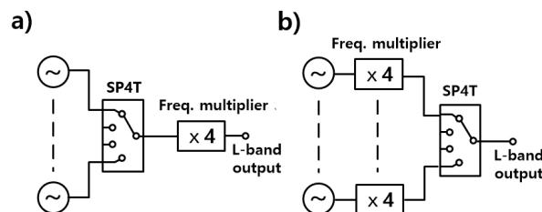
**Figure 1.** Block diagram of analog direct frequency synthesizer.
