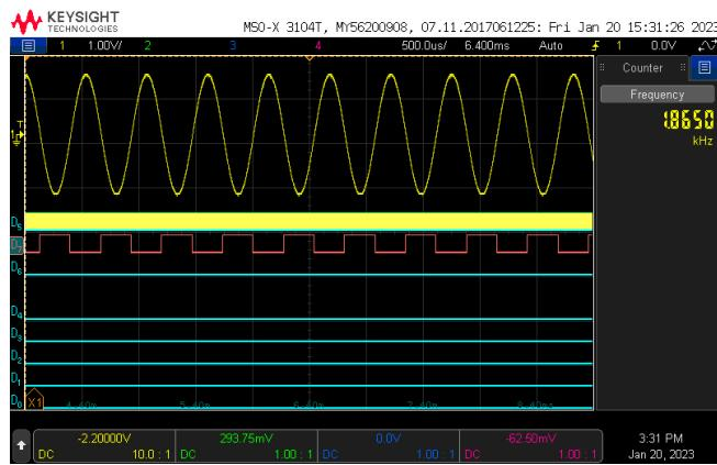
**Figure A12.** Upper frequency 1865 Hz generated waveform.
