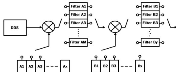
**Figure 6.** Conceptual diagram of DAFS with DDS added.
