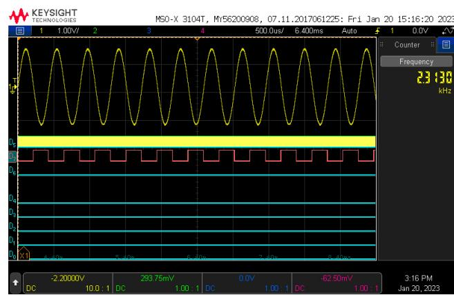
**Figure A2.** Upper frequency 2313 Hz generated waveform.
