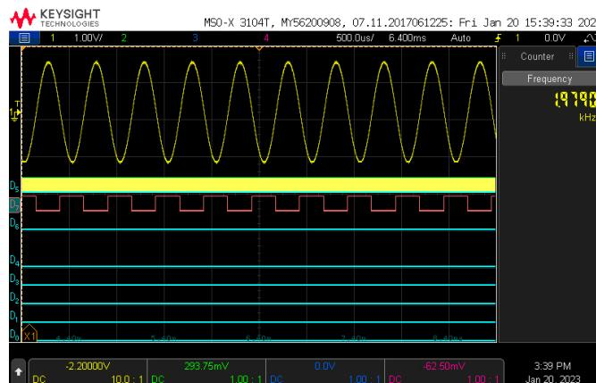
**Figure A3.** Lower frequency 1979 Hz generated waveform.
