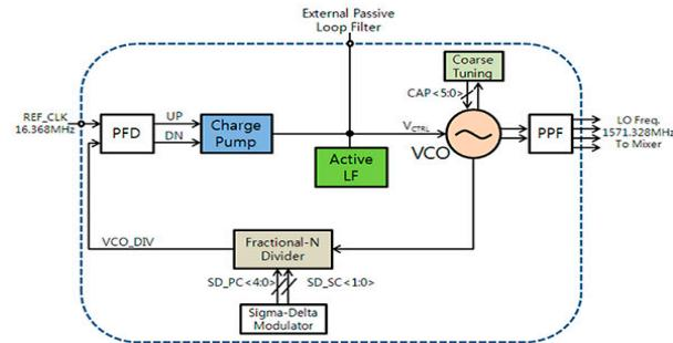
**Figure 3.** Application structure of PLL frequency synthesizer.
