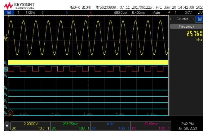
**Figure A5.** Lower frequency 2576 Hz generated waveform.
