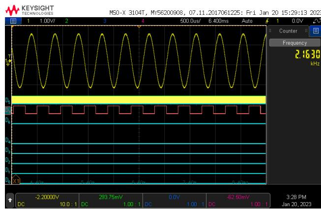
**Figure A10.** Upper frequency 2163 Hz generated waveform.
