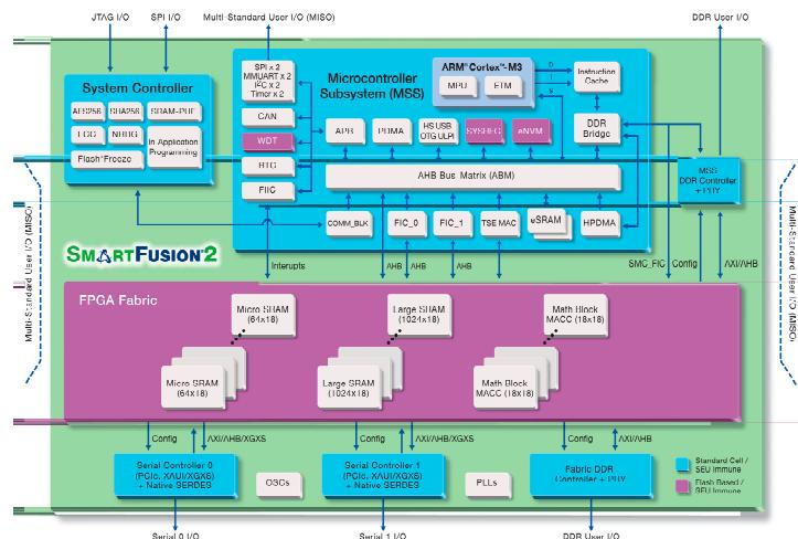
**Figure 25.** Internal block diagram of M2S010.
