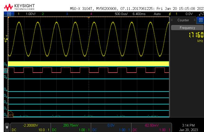
**Figure 29.** Upper frequency 1716 Hz generated waveform.
