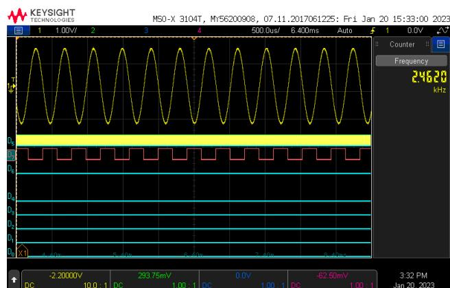
**Figure A14.** Upper frequency 2462 Hz generated waveform.
