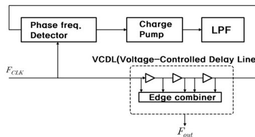
**Figure 4.** Frequency synthesizer block diagram based on DLL.
