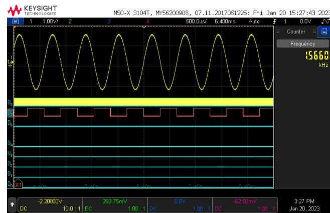
**Figure A8.** Upper frequency 1566 Hz generated waveform.
