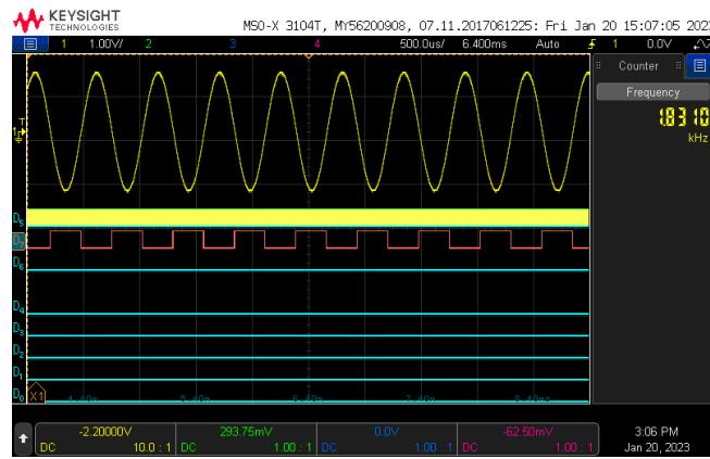
**Figure A11.** Lower frequency 1831 Hz generated waveform.
