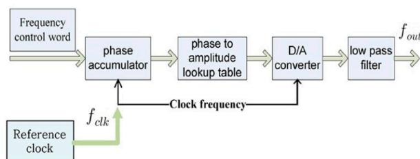
**Figure 5.** Direct digital frequency synthesizer basic diagram.
