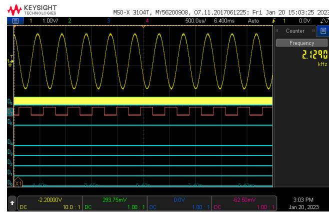
**Figure A9.** Lower frequency 2129 Hz generated waveform.
