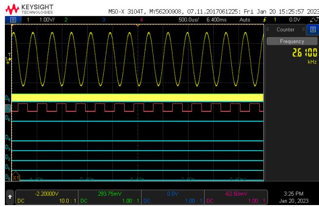
**Figure A6.** Upper frequency 2610 Hz generated waveform.
