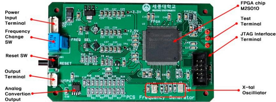
**Figure 26.** Circuit board used for testing.
