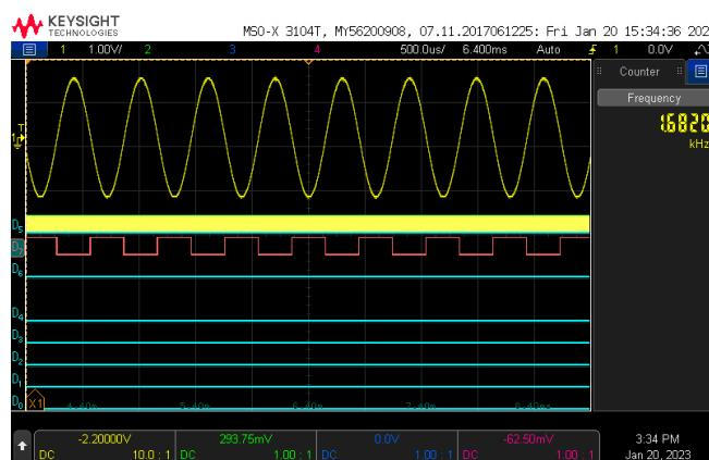
**Figure 28.** Lower frequency 1682 Hz generated waveform.
