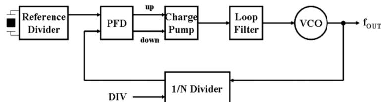
**Figure 2.** Basic structure of PLL frequency synthesizer.
