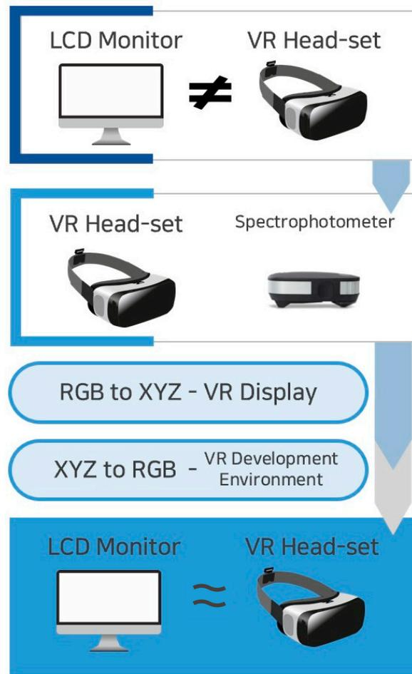
Figure 10. Color matching with a design display through the characterization of VR displays.
