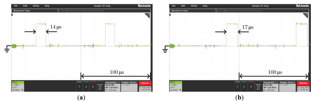
**Figure 11.** Experimental results of computational time consumption with different controls. (a) PI controller (b) Proposed method.
