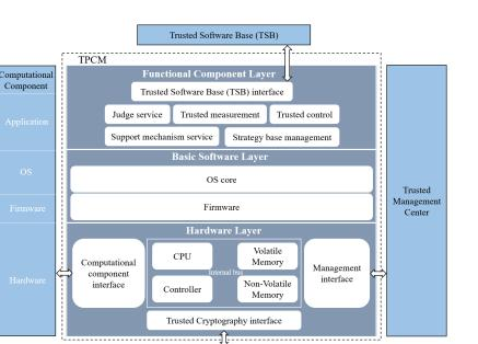
Figure 5. The function and interface framework of TPCM.
