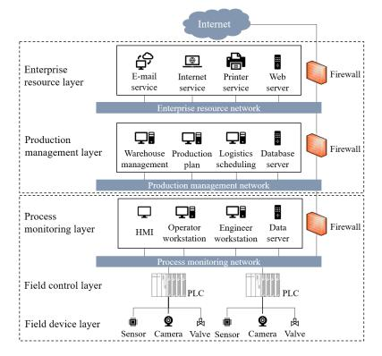
Figure 1. The typical architecture of industrial control systems.
