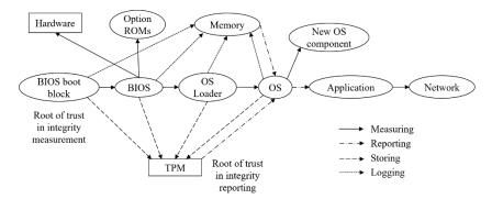
Figure 3. The chain of trust of TC group trusted PC.
