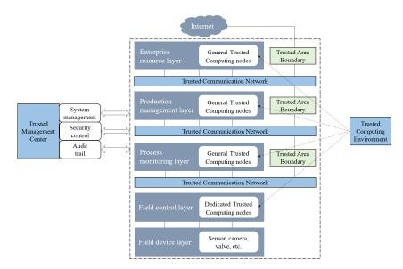
Figure 6. An active defense security structure for industrial control systems.
