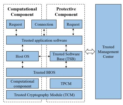
Figure 4. Dual architecture supported by TC 3.0.
