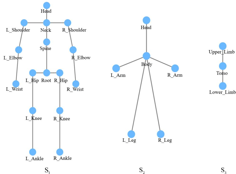
**Figure 6.** Description of the structure of the body joints and its sub-structures. We designed these pre-defined structures to retain the physical human topology.
