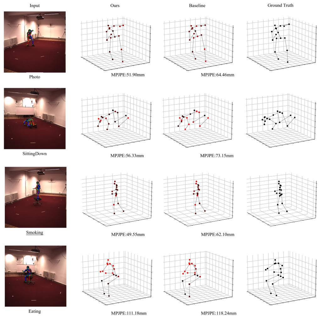
**Figure 13.** Qualitative comparisons between our proposed method and a baseline method [3] on challenging poses in the Human3.6M [25] dataset. The 2D keypoints detected by the CPN [31] were used as the input samples, and the brightness of points represents the scale of the error, amplifying the visual discrepancy from the ground truth.
