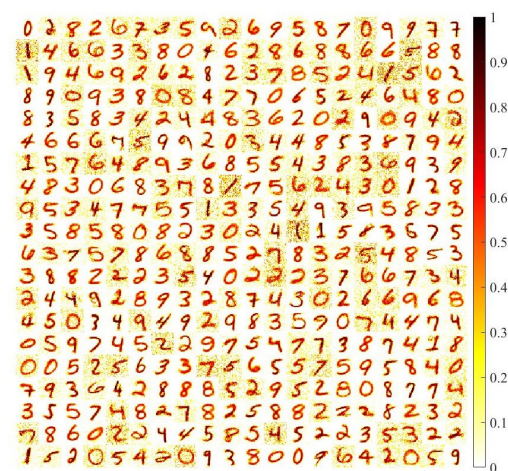
Figure 9. Synaptic weight matrix after training completion. The excitatory neuron layer comprises 400 neurons arranged in a 20 \times 20 grid. Each neuron is fully connected to 784 input layer neurons through synaptic connections. The synaptic weights, totaling 784, are rearranged into a 28 \times 28 grid, resulting in the weight distribution. The white color represents the minimum weight value of 0, while the black color represents the maximum weight value of 1.
